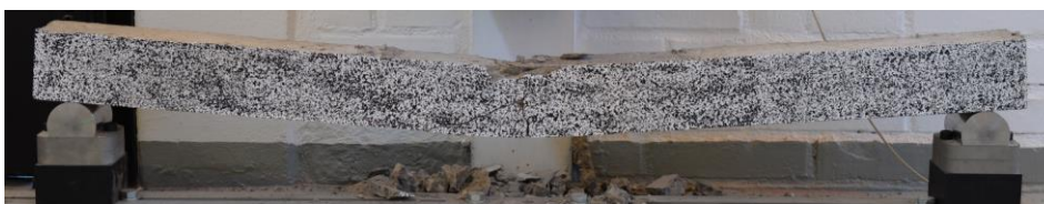
Figure 10.15 Beam 12 after impact from 4 m.
