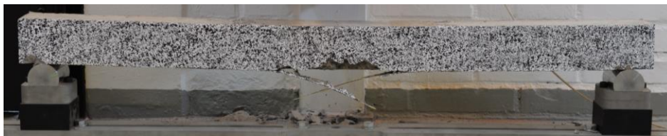
Figure 10.14 Beam 13 experiencing partial rupture of FRP.
