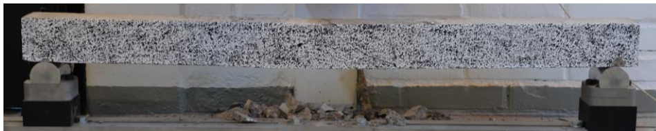
Figure 10.11 Beam 14 showing cone-like shear cracks under the impact area.
