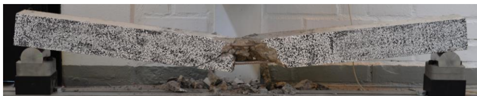
Figure 10.16 Beam 18 after impact from 5.7 m.
