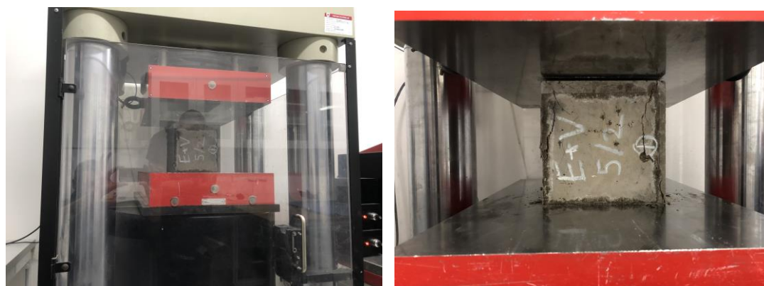
Figure 8.16 Test of cube compressive strength.
