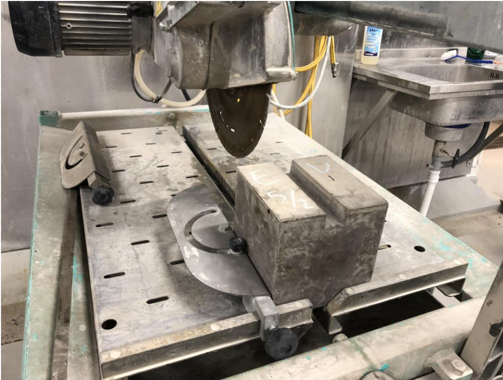
Figure 8.17 Preparation of the specimen and the sawing of the starting notch.
