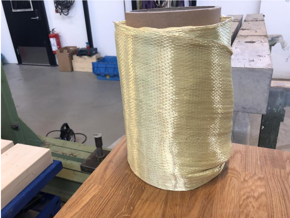
Figure 8.7 The kevlar used to strengthen the beams.
