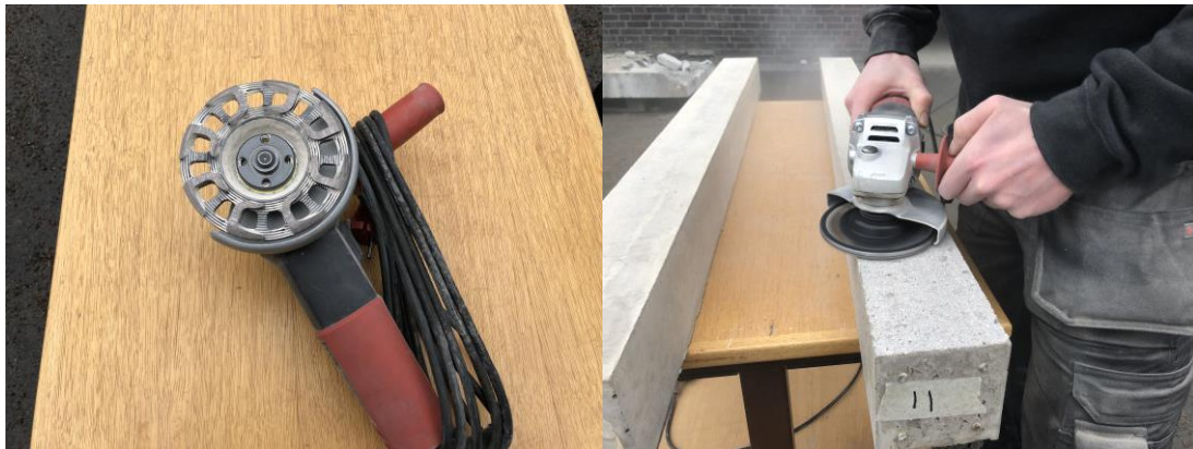
Figure 8.5 Tool and set-up for grinding surfaces of specimen.
