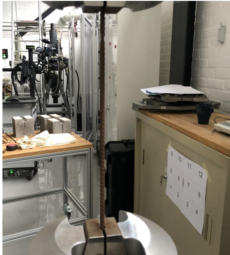
Figure 8.19 Tensile test of reinforcement bars.
