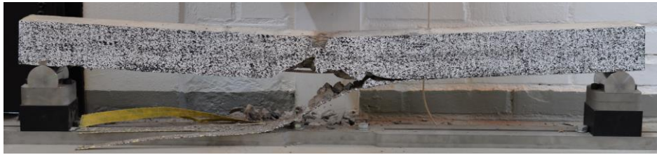
Figure 10.13 Beam 09 showing cone-like shear cracks under the impact area causing debonding. Similar to the failure mode described as intermediate flexural-shear crack induced interfacial debonding.
