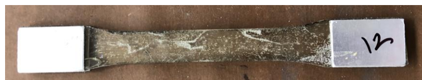
Figure 8.21 Test specimen with aluminium plates attached.
