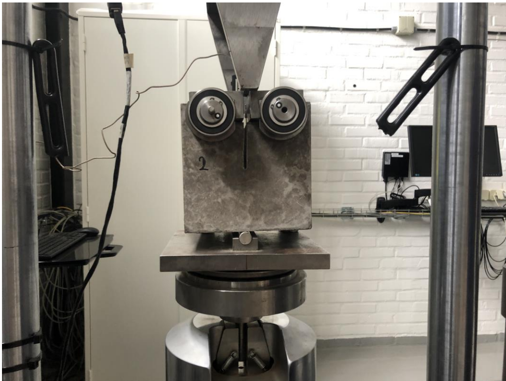
Figure 8.18 Wedge splitting test set up.
