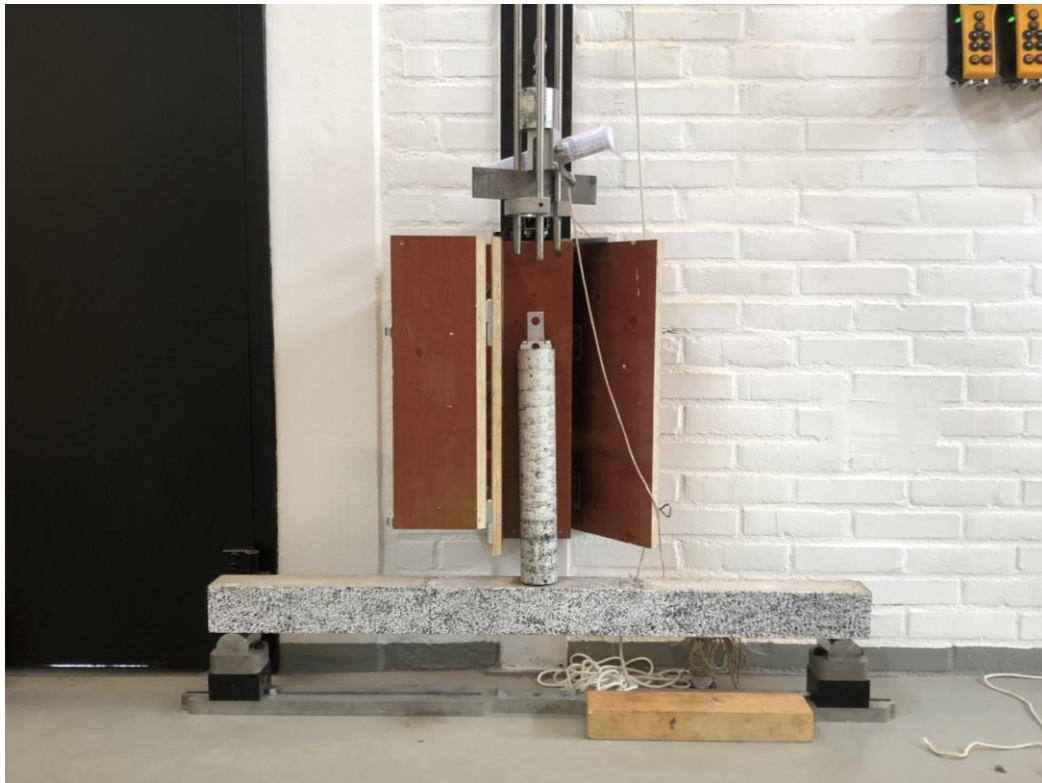
Figure 8.23 Test set-up for dynamical tests.
