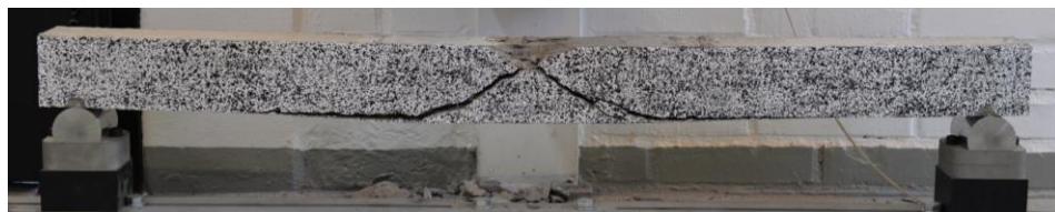
Figure 10.12 Beam 22 showing cone-like shear cracks under the impact area to a more severe degree.
