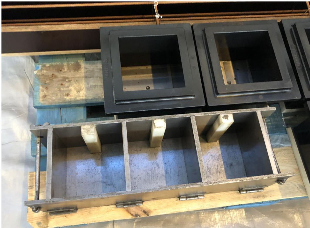
Figure 8.3 Moulds for the material tests of concrete. Compressive strength test at 28 days and during the day of testing of the beams as well as cubes for WST.
