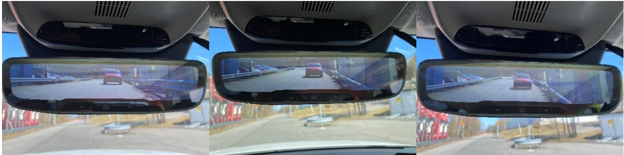
Figure 27 - Images of the display view from the bumper, glass and roof position at zoom level 2.5 (from left to right).
