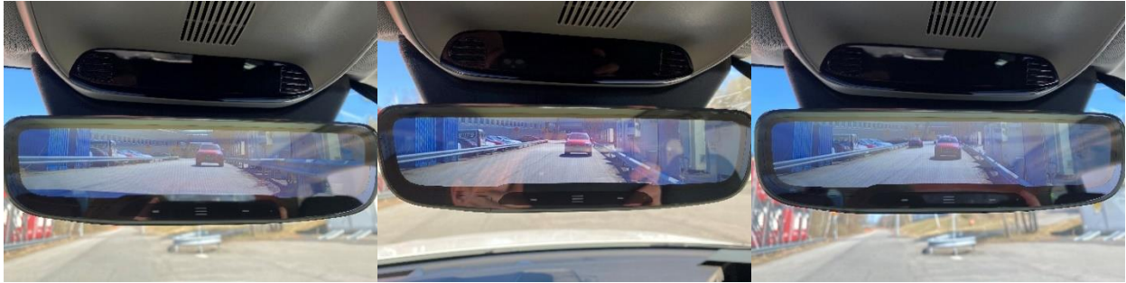
Figure 26 - Images of the display view from the bumper, glass and roof positions at zoom level 2.0 (from left to right).
