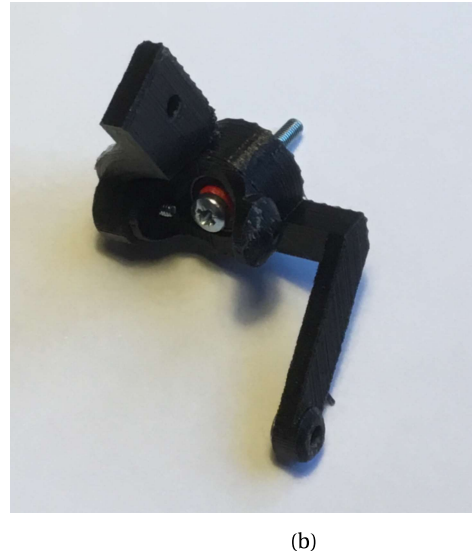
Figure 5: a) Right wheel holder with the direction of the screw b) Illustration of right front wheel.
