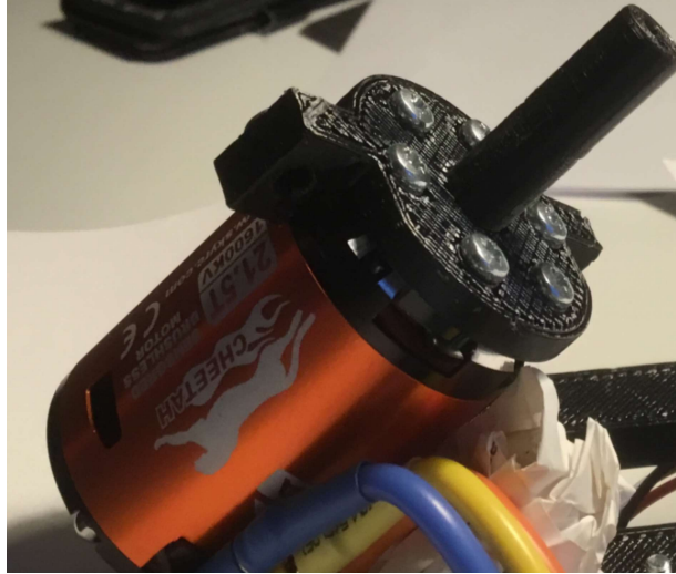
Figure 9: Brushless motor with motor holder and the shaft connector.
