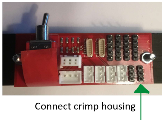
Figure 37: Where to connect crimp housing from Raspberry Pi to daughter board.
