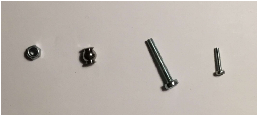
Figure 51: From left to right, screw nut, hollow ball, screw (4.3x21), screw (2.3x13)
