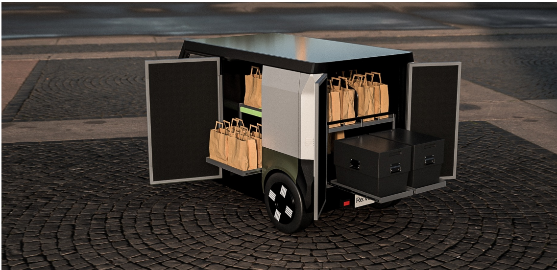
Figure 6.4: Rendering of Re:Volt with one side door and both rear doors opened, with three lower shelves in extended positions.
