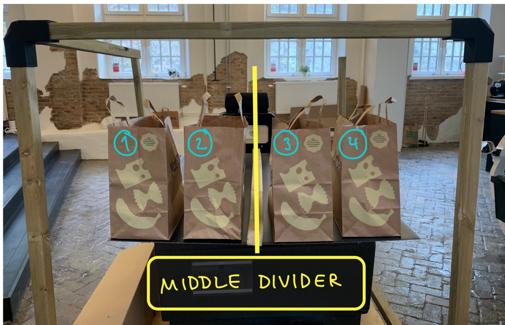
Figure 5.25: Physical test and overlaid sketches to visualise the implementation of a divider in the middle of the upper shelf, seen from the back of the cargo space.
