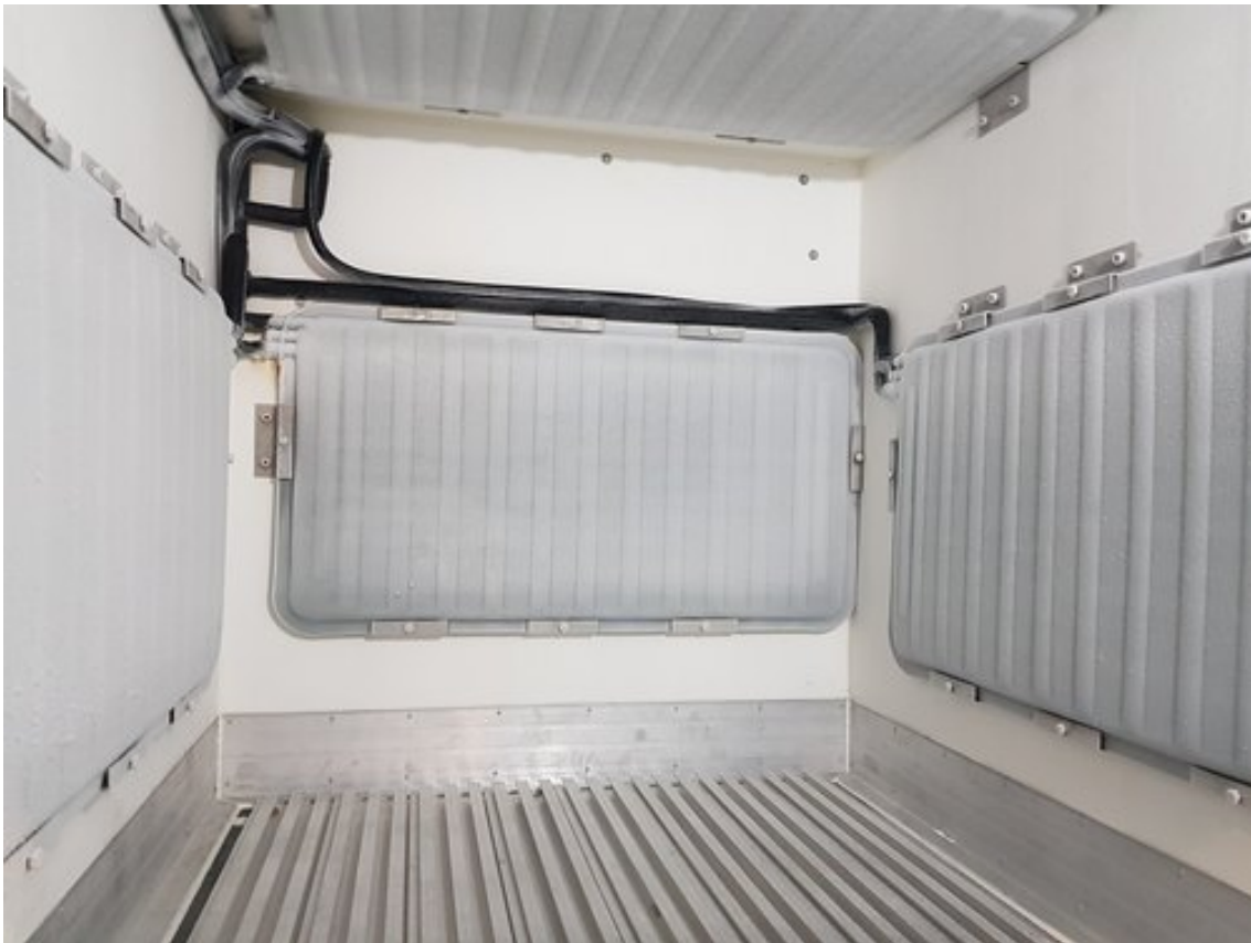
Figure 2.2: An example installation of active eutectic plates in a cargo space, from IndiaMART (n.d.).
