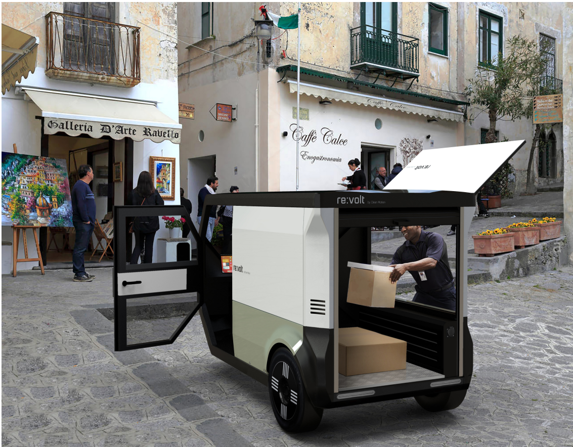
Figure 4.34: The initial design of Re:Volt with static, lower side panels visualized in green.
