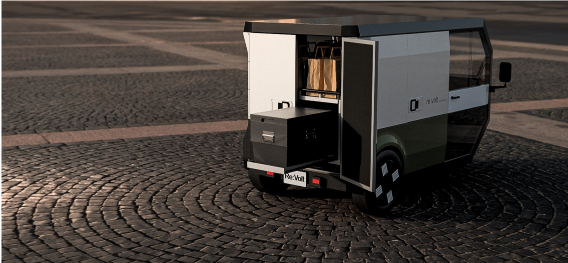
Figure 6.2: Rendering of an alvobox that has been pulled out from the rear of Re:Volt.
