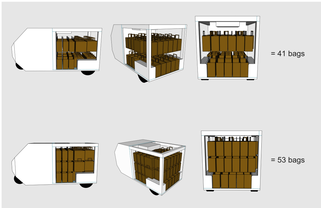
Figure 4.20: Comparison of how two or three levels of shelves carrying paper bags would fit inside the cargo space of Re:Volt.
