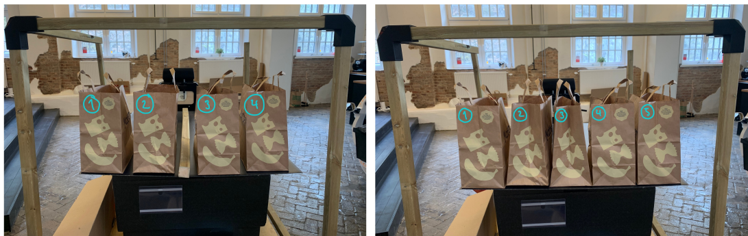
Figure 5.23: Physical test of implementing four and five rows of paper bags on the upper shelf together with a full scale mock-up of Re:Volt and a representation of the shelf structure concept with similar dimensions.
