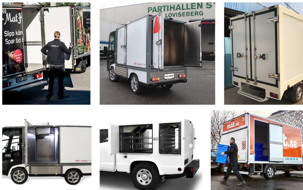
Figure 5.4: Different doors to a cooled cargo space.
