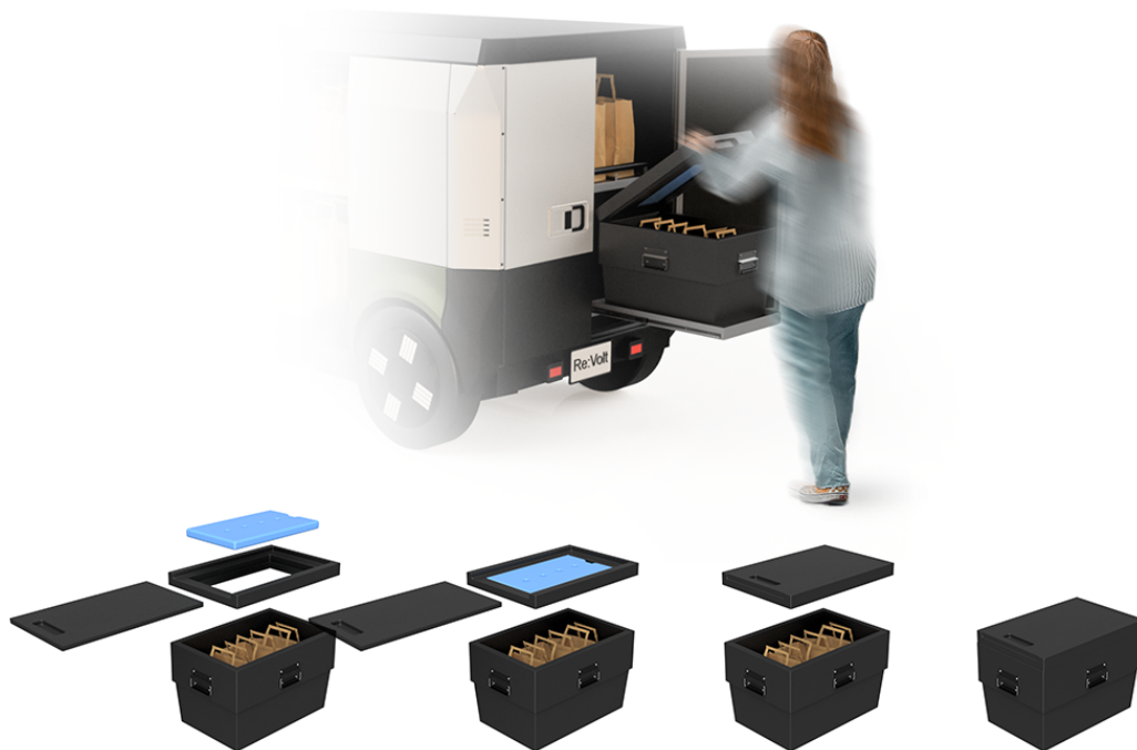
Figure 6.14: Illustration of how the alvobox can be opened during a delivery (top) and a sequence of how the PCM block is inserted into the lid of an alvobox.
