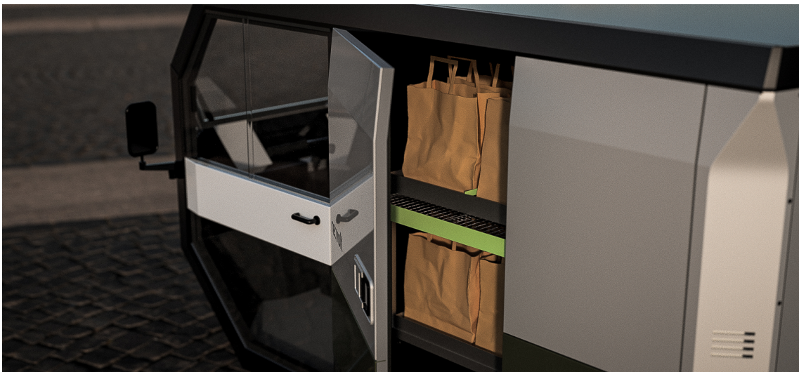
Figure 6.3: Rendering of an opened side door of Re:Volt, showing the upper extendable shelf in a pulled out position.
