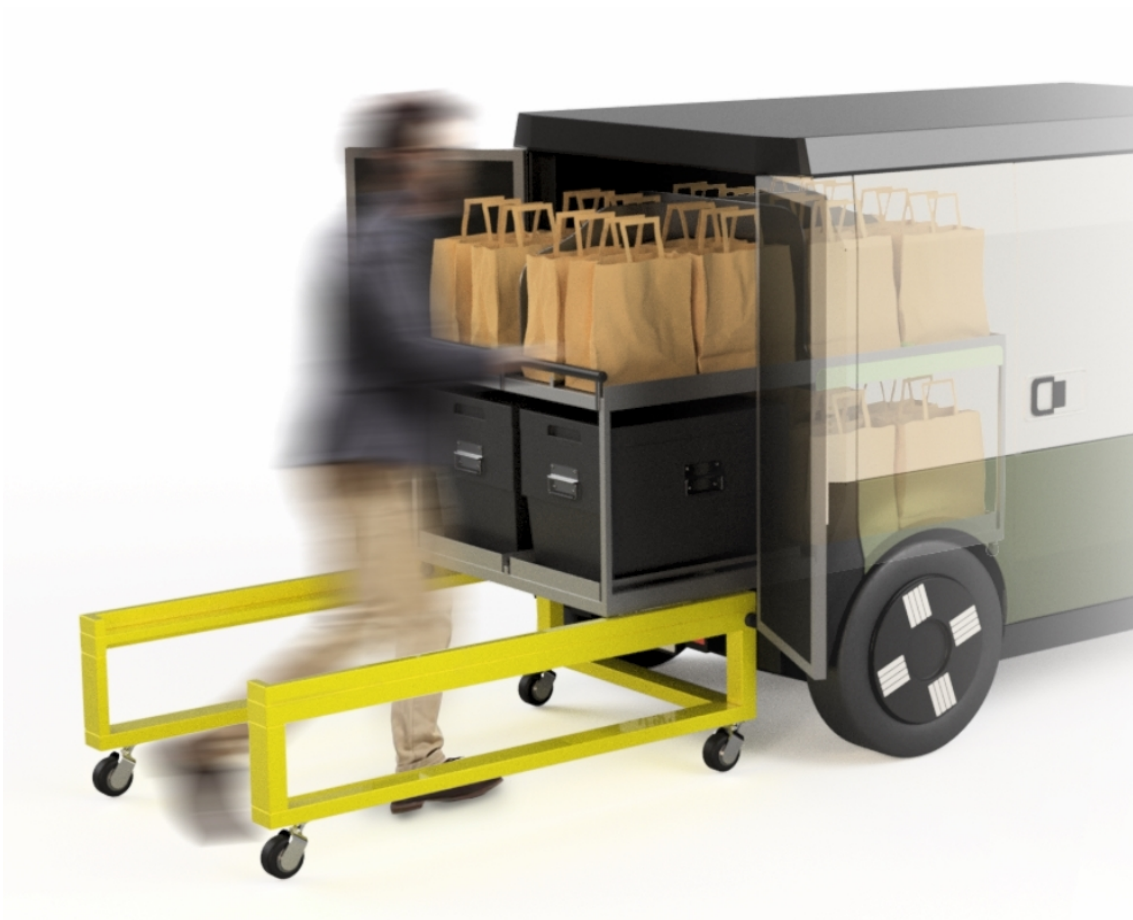
Figure 6.19: A fully loaded Re:Load pushed into the cargo space using the transportation dolly.
