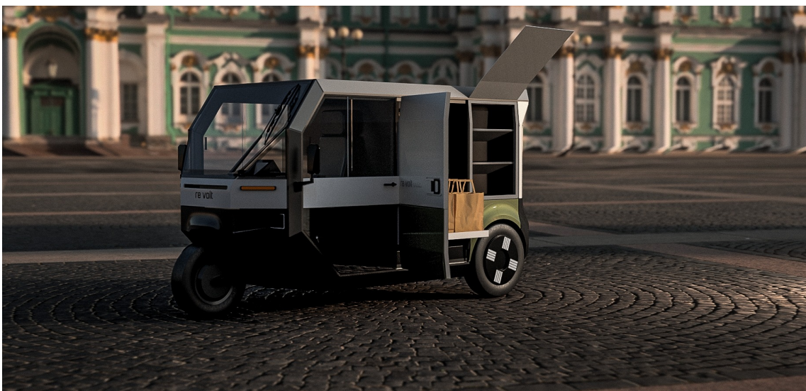
Figure 6.5: Rendering of Re:Volt that showcases the compartment located above one of the wheelhouses.
