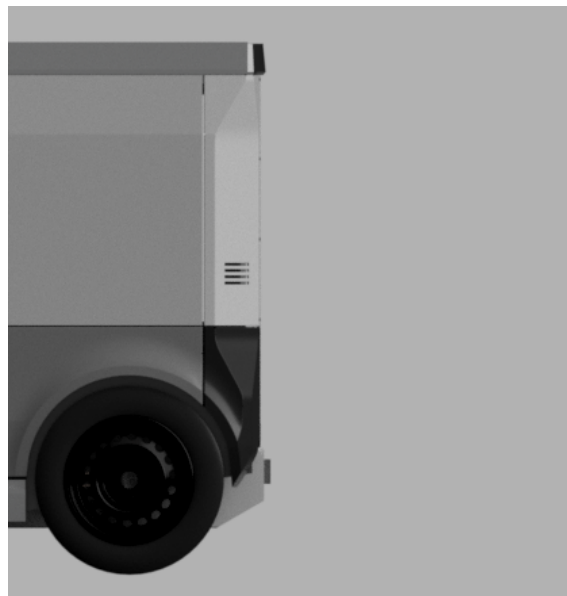
Figure 5.31: Rear edge of the cargo space shaped like a large chamfer, affecting the design and placement of the insulating panels part of insulating the cargo space.
