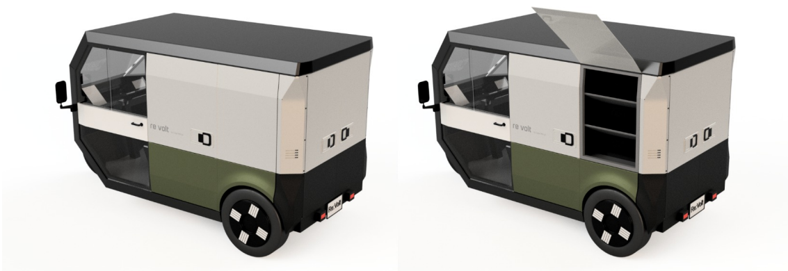
Figure 6.22: Storage compartments located above the wheelhouses in Re:Volt, accessed from the sides of the cargo space.
