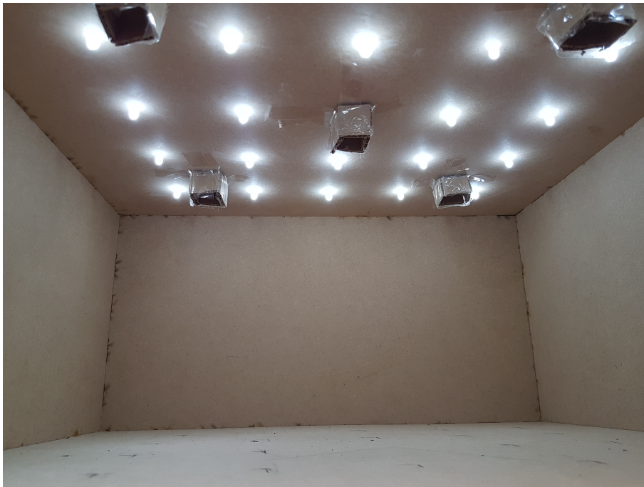
Figure 3.3: Inside of the MIMO system, with the LEDs visible, the sensors are placed inside the cardboard screens
