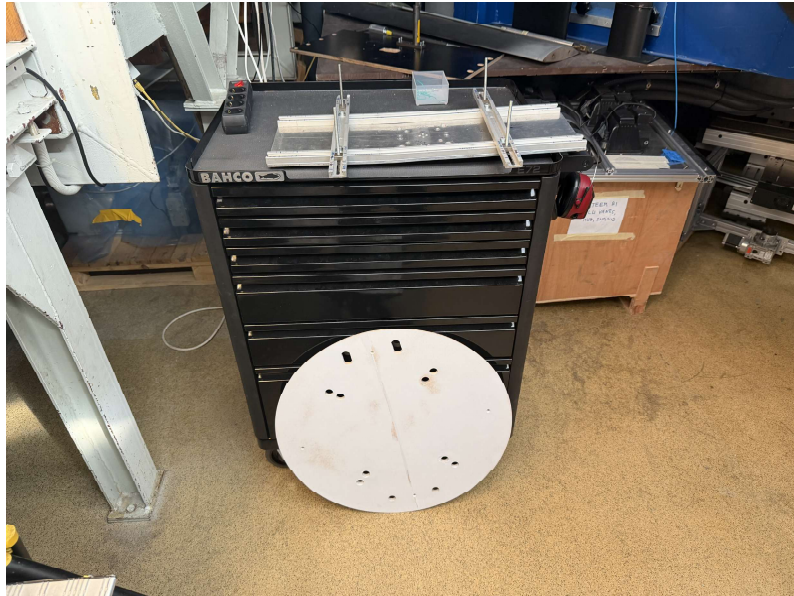
Figure 3.28: Custom mounting platform and jig used to secure the scale model in the wind tunnel.
