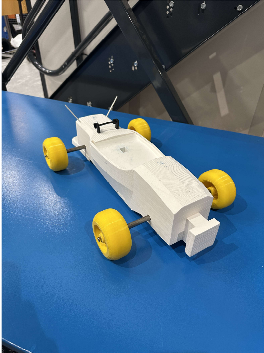
Figure 3.25: A view of the half-completed 3D-printed car. In this state, the car is missing the sidepods, both wings and the optional driver.
