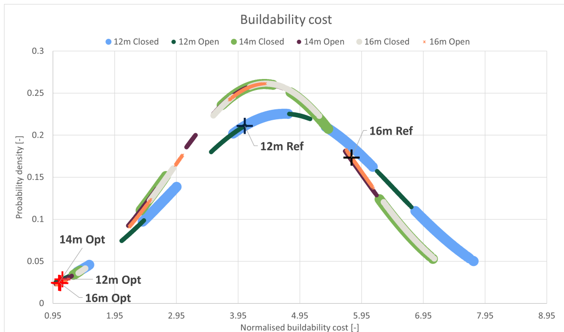
Figure 4.12: Probability density vs. Normalized buildability cost per span and reference bridge. Most optimized bridges are based on equivalent cost marked with red crosses.
