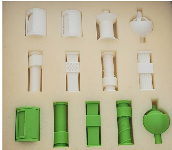
Figure 4.2: Polymer prototypes of regular joints (green) and redesigns (white), made with Fused Deposition Modeling
