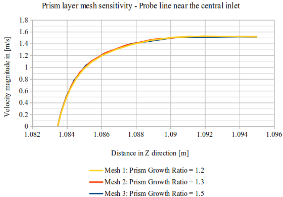
Figure 5.2: Velocity gradient captured by the prism layer mesh at a probe line 15 cm away from the central air inlet
