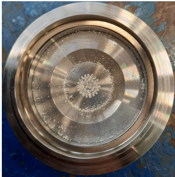
Figure 5.10: DLPI component showing excess material spilled over from measurements
