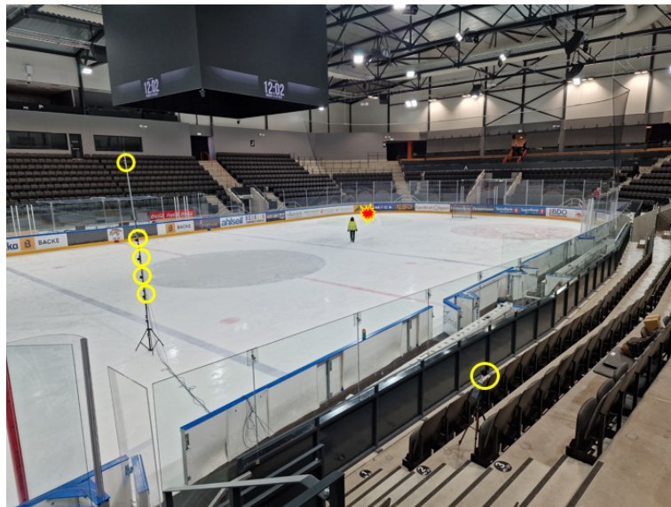
Figure 3.2: First reverberation time measurement setup. Receiver positions are marked with yellow and source position is marked with red
