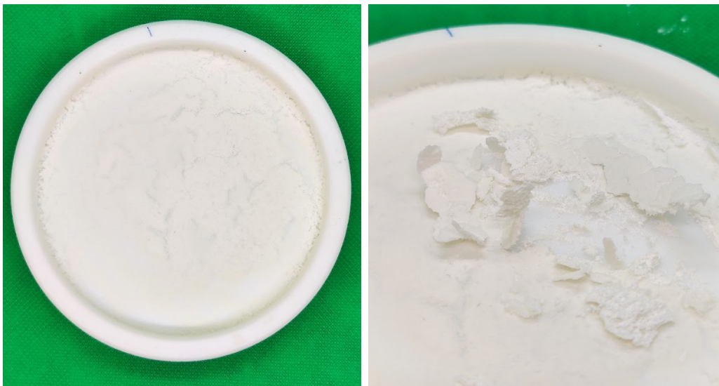
Figure 4.8: A3 as a cured film on a Teflon-mould. The uneven surface on the picture to the right is caused by scraping of a spatula.
