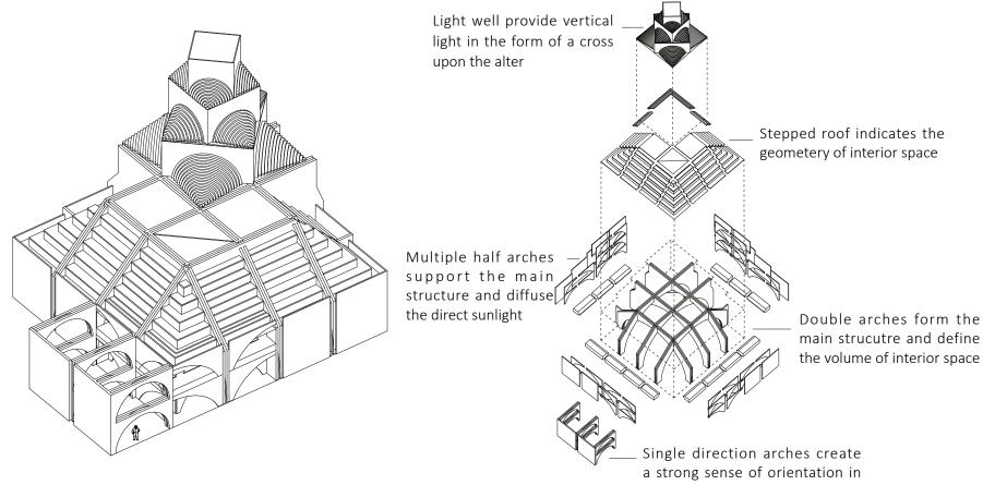
The Christ Church contains five parts - entrance aisle, enclosure walls, main structure, roof and light well. Arches as the main structure system have both structural and spacial roles. The strucutre as the space-defining elements creates space with strong sense of centrality, isolation and calm.
