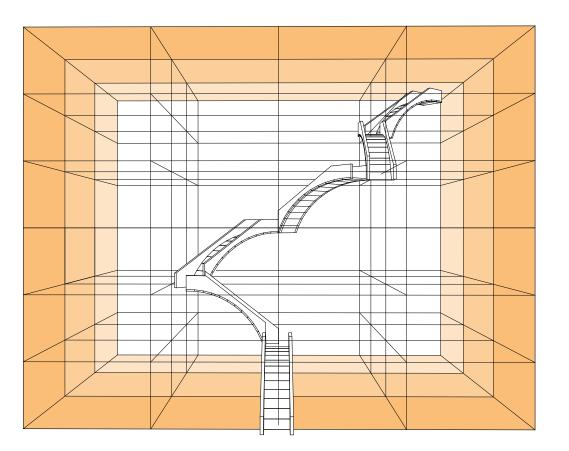
The arches work as the bearing system in the project and half arches work as stairs that connect the normal levels and one third levels. And the position of stairs is dominated by the performance of arches. The diagram shows that stairs can develop in different directions between arches and also form the vertical circulation
