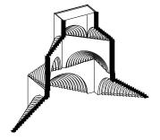
The spalyed valts offer a solution to balance different geometries and provide direct sunlight for inner space
