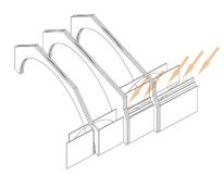
Multiple half arches work as curtains and diffuse the daylight
