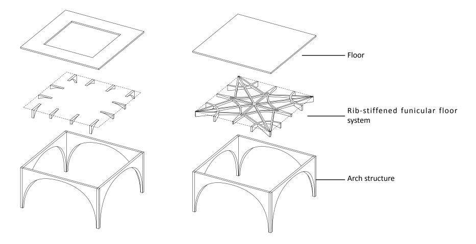
Developed from the floor system, a new system is introduced between floor and arch. These tiny arches dispense and transmit the strength. This system shows the ability of arch on different scale. 4.4 Refining arches based on the mechanical property and introduce the one third level
