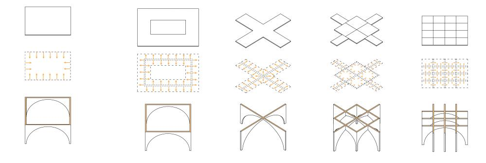
Independent arch can not give enough support foece to the center of floor slab, which means the slab have to bear the load itself The size and position of floor slab is dominated by the performance of arch, and the arches will always be the primary bearing system. Therefore the performance of arch is not only influence people's perception in the space, but also influence people's movement on the upper level
