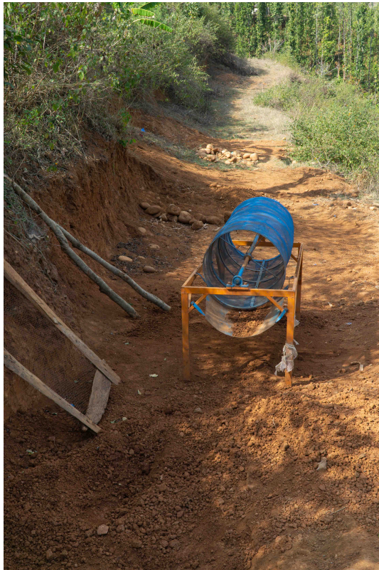
(a) Soil procurement and soil sieving machine.
