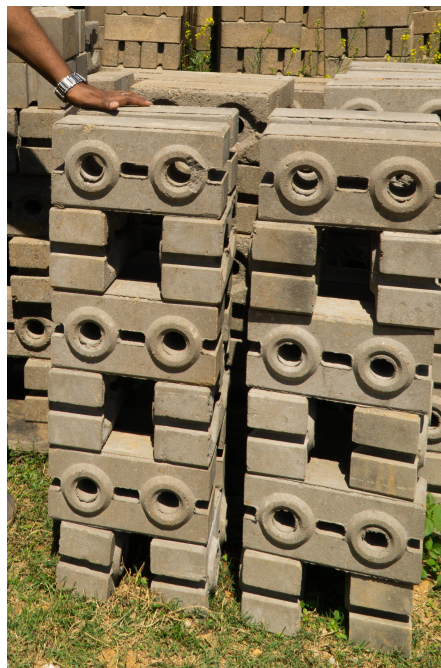
Figure 6.4: Stack of CSEB units curing/drying in field in Jajarkot.
