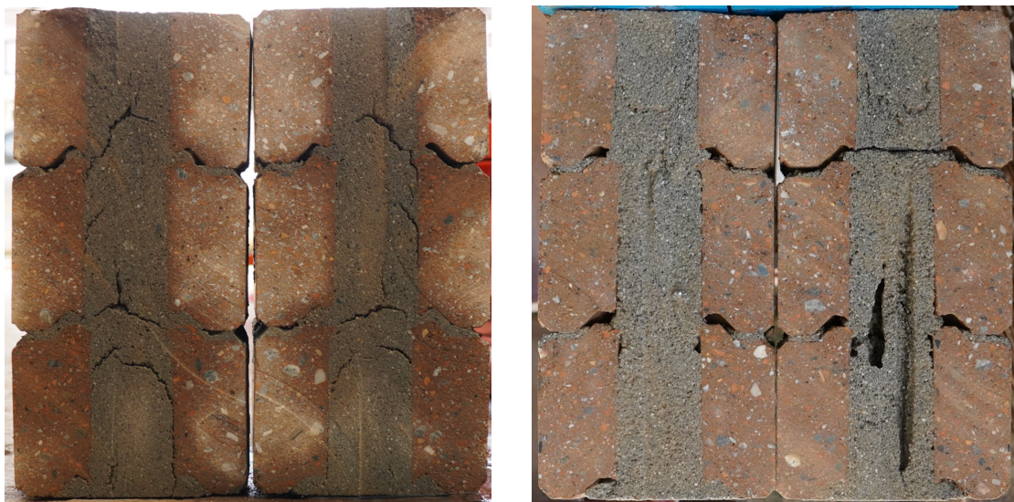
Figure 8.1: Block cut without being tested. 1:3 grout mix left and 1:6 grout mix right.
