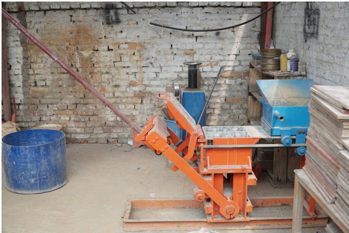
Figure 6.3: Interlocking Compressed Stabilised Earth Block machine built and produced by BUN.
