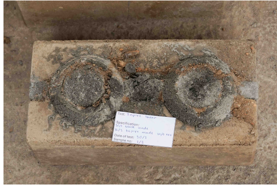
Figure 7.10: View of the grout key formed within the interlocking void post testing.
