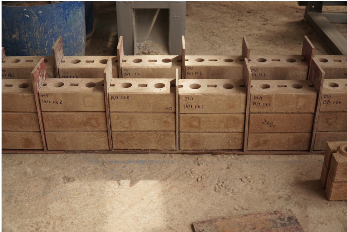
Figure 6.5: Triplet specimen production with phenolic coated plywood between triplets.
