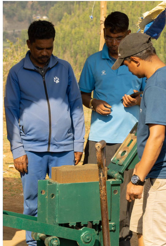
(b) Block pressing machine with block being pressed.
