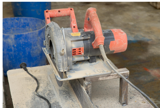
Figure 6.13: Stone cutter and setup used for block sectioning.
