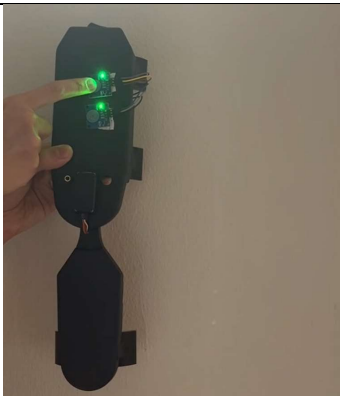
Figure 4.6: First part of the exoskeleton motion. Pressing and holding the touch sensor to initiate the 0-to-90-degree motion of the exoskeleton.
