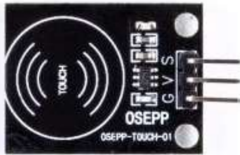
Figure 2.4: The Touch Sensor model used to control the exoskeleton arm, from the... [8]
