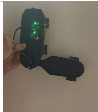
Figure 4.8: Third part of the exoskeleton motion. The arm reaching the desired joint angle of 90 degrees.
