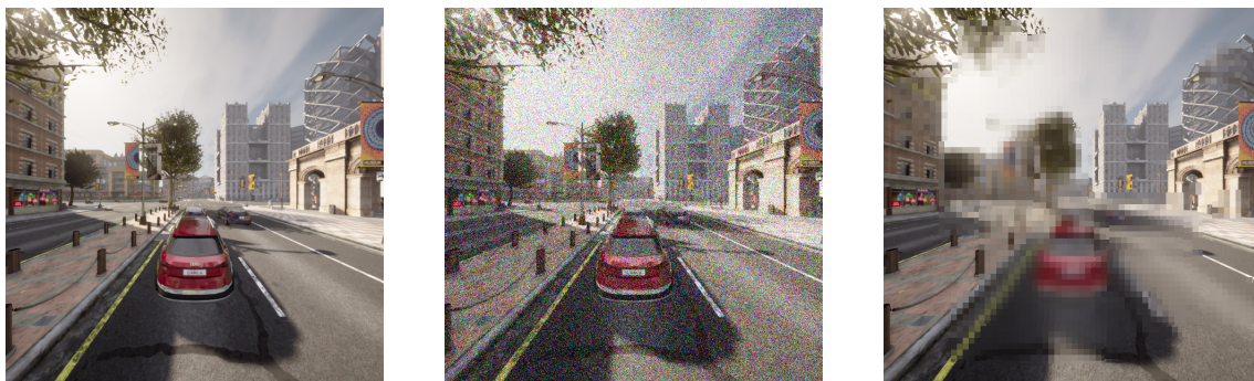
Figure 3.4: Comparison of Original Image (left) with Gaussian Noise (center) and Mosaic Noise (right)
