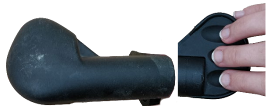
Figure 13, Seat height control
