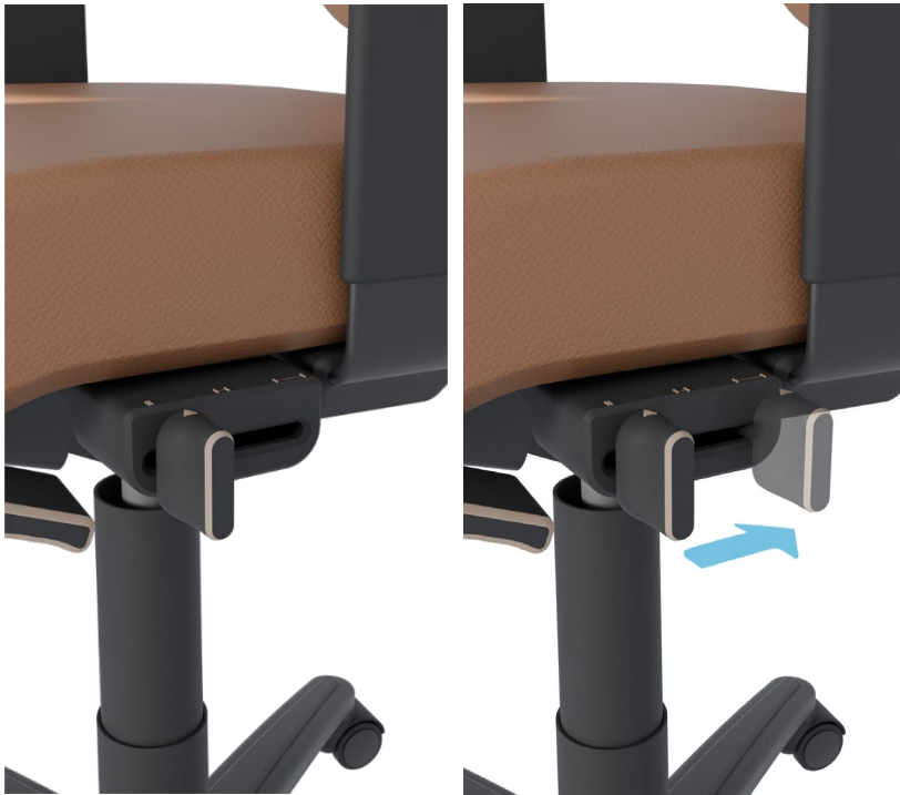
Figure 51, Illustrated sliding movement of the seat position control
