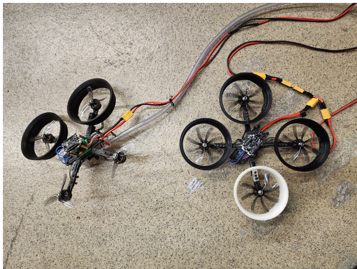
Figure 3.36: Tethering system with tube connected
