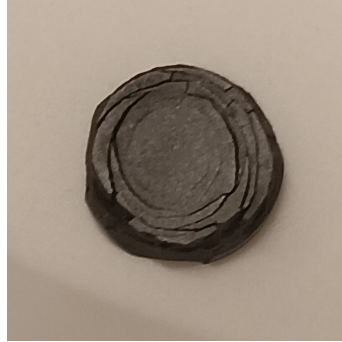
Figure 4.3: The "underside" of pellet B1 after sintering three times.
