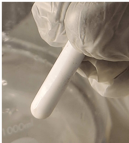
Figure 4.22: Magnetic stir bar used for the precipitation. A flat surface has formed on one part of the bar.
