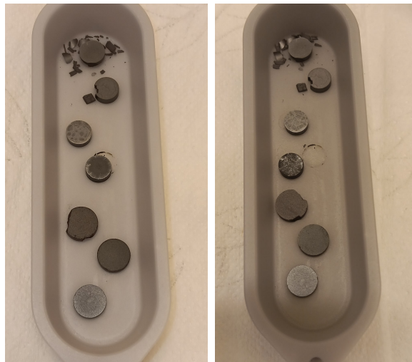
Figure 4.2: All seven pellets (from top to bottom: B1-B4, R1-R3) after the second sintering (left) and after the third sintering (right).
