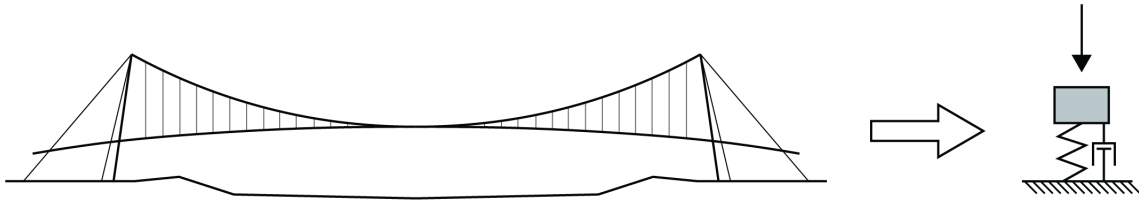
Figure 3.2 Equivalent SDOF oscillator for one natural frequency corresponding to one vibration mode of the structure (JRC, 2009)
