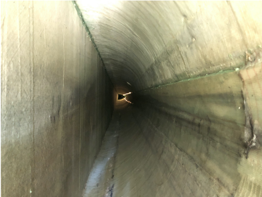
Figure L.4 Interior of the blade, web and leading edge (own photo).
