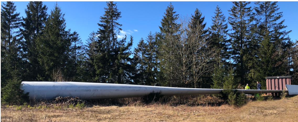
Figure 4.1 Decommissioned NWP28.3 ATV blade near Halmstad, Sweden
