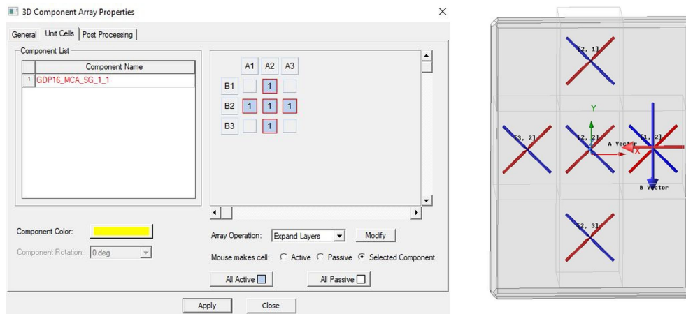
Figure 2.4: HFSS Array Tool interface demonstrating multiple component array configuration for systematic antenna array modeling.
