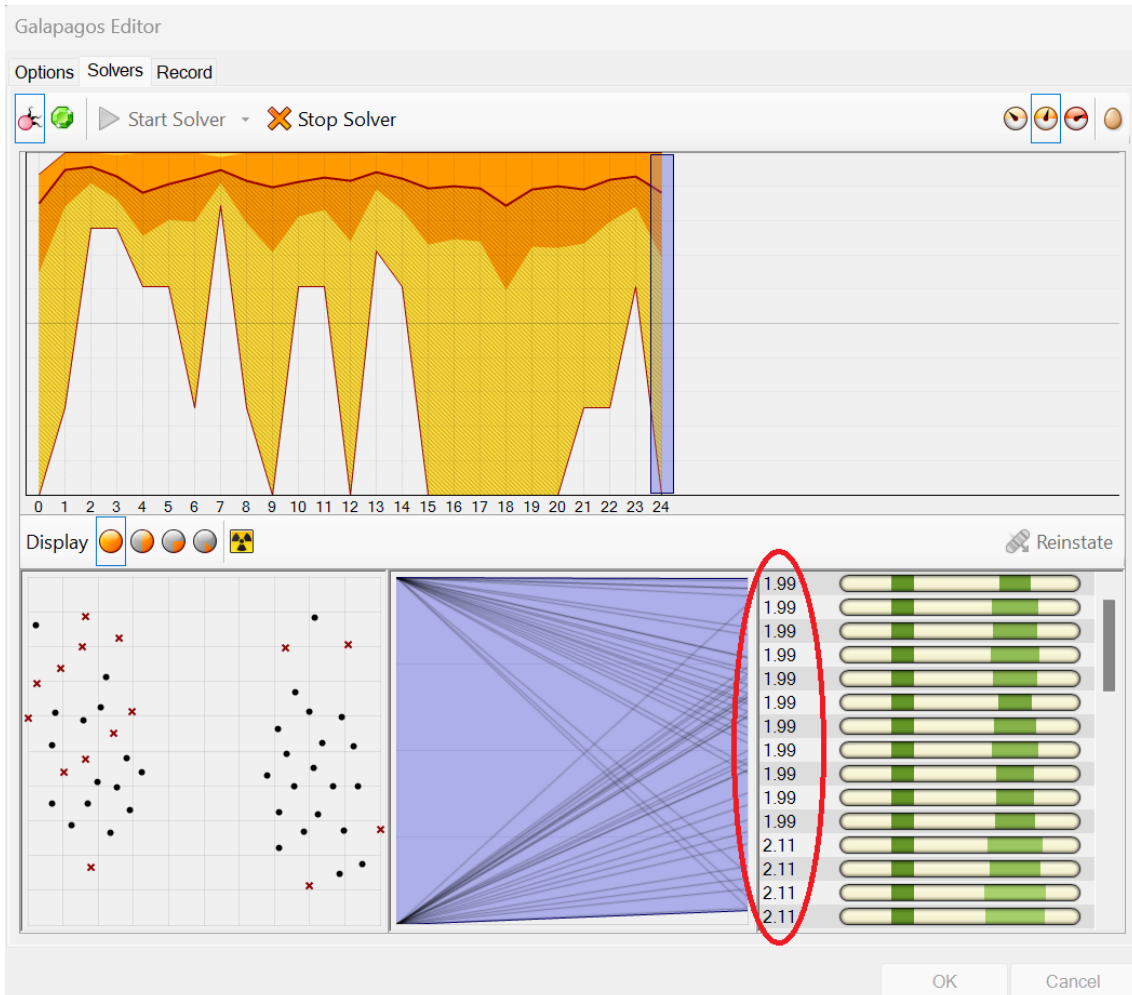
Figure A.9: The solver window while the optimization is run. Here the values have converged.
