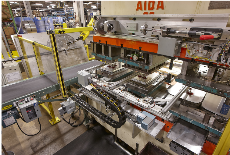
Figure 4.1: Stamping tool mounted inside press
