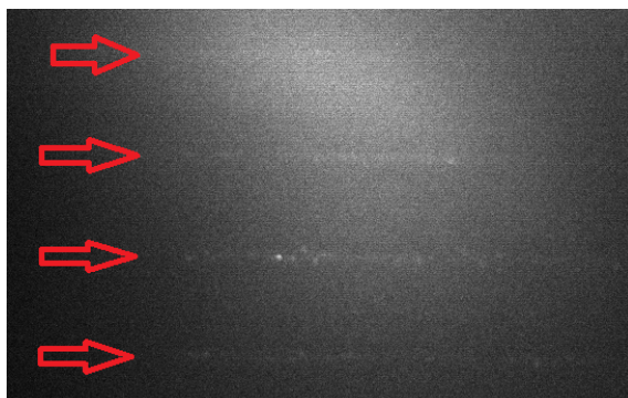
Figure 4.9: An image where a SNARF-1 dilution with the concentration 100 \mu\text{g}/\text{ml} is imaged with no dispersion, \text{RPA} = 180 . The arrows indicate the location of four nanochannels, barely visible over the background.
