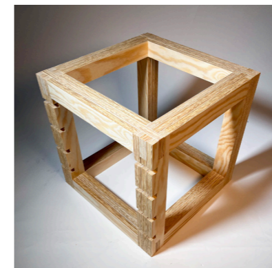
Pine wood structure assembled without any fasteners or adhesives.
