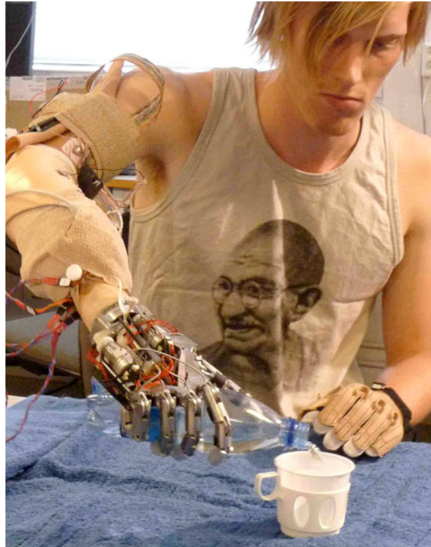
Figure 2.2: One of the patients from the SmartHand project testing the hand. Picture taken from [12], used with permission.
