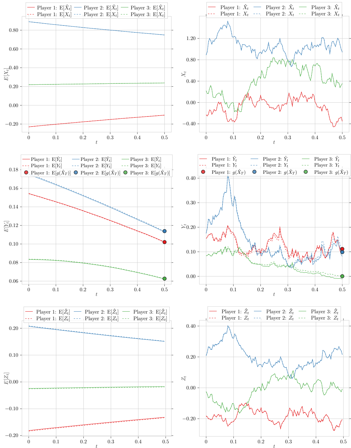
Figure 6.1: Numerical results for the Deep fictitious play method for d = \ell = 1 with three players. Columns represent the expectation and one representative trajectory, respectively. The rows represent the different processes. Each color represents a different player. The solid line represents the approximation of the process, and the dashed its analytical counterpart.
