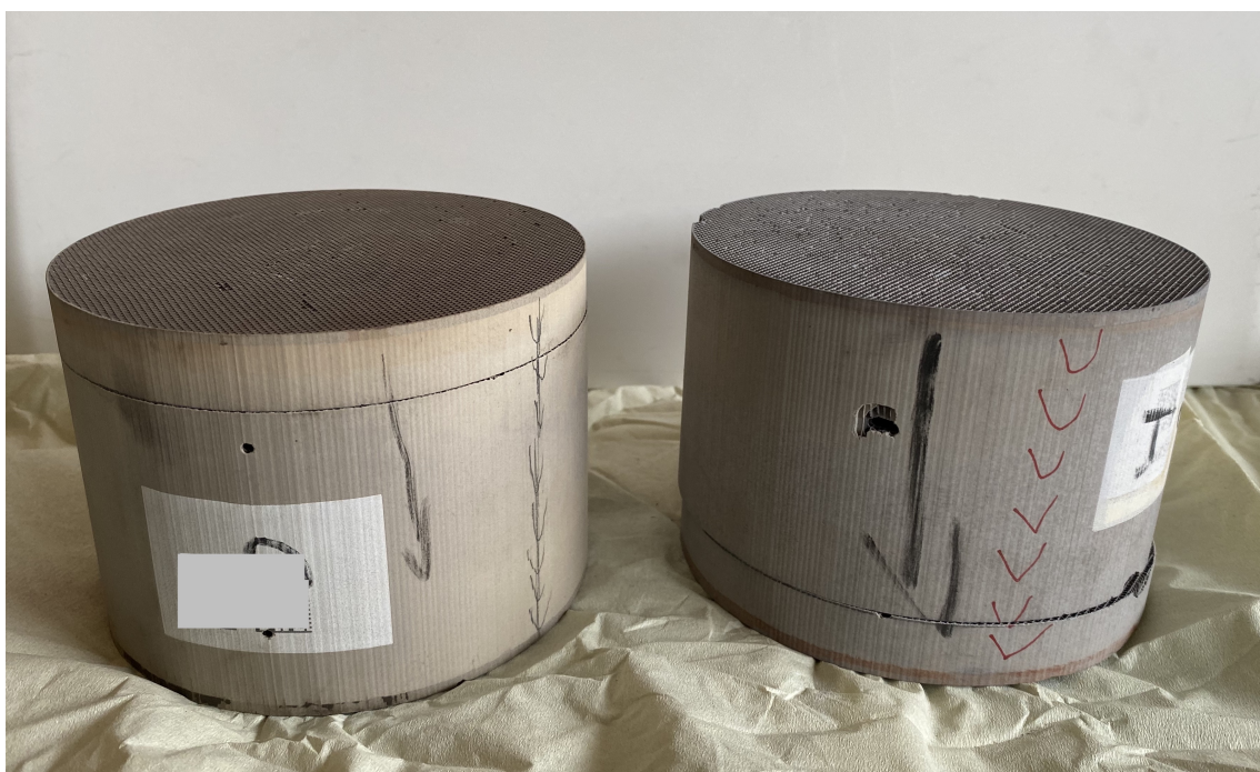
Figure 3.1: The two catalyst bricks supplied from Aurobay, stabilised to the left and the bench aged brick to the right.
