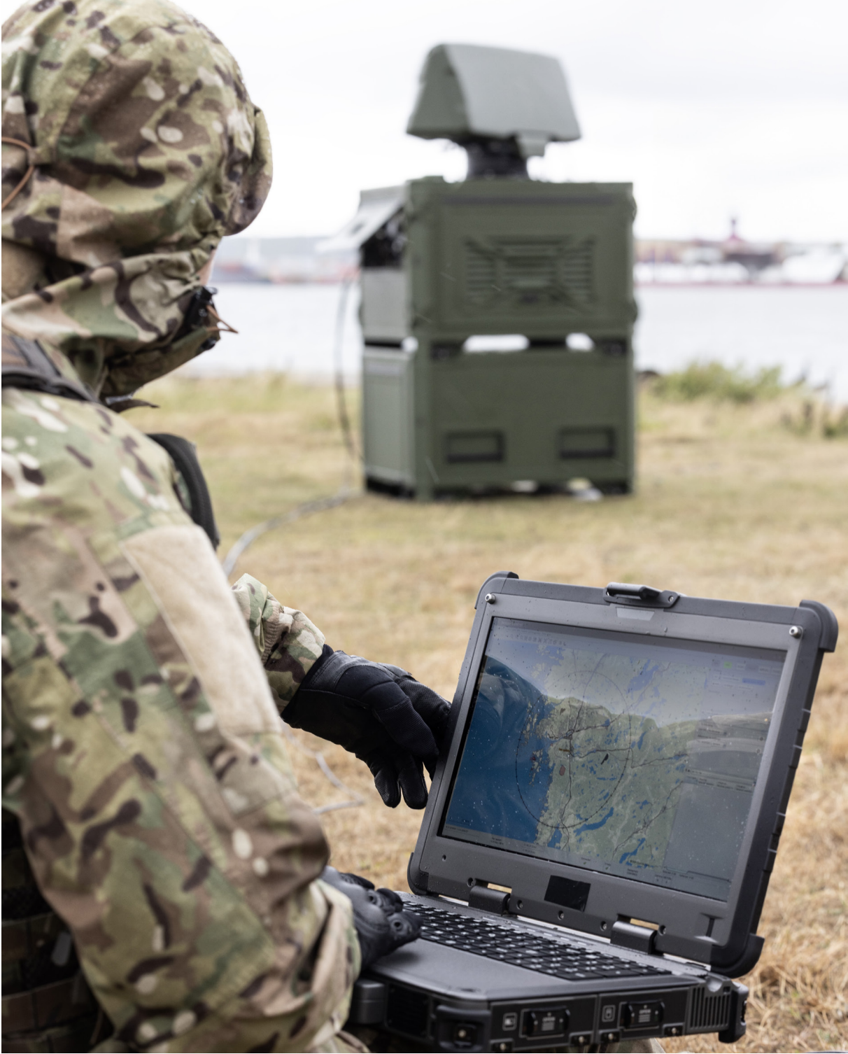
Note. Photograph of the Giraffe 1X mobile radar system. (Saab AB, 2023). © Saab AB.
