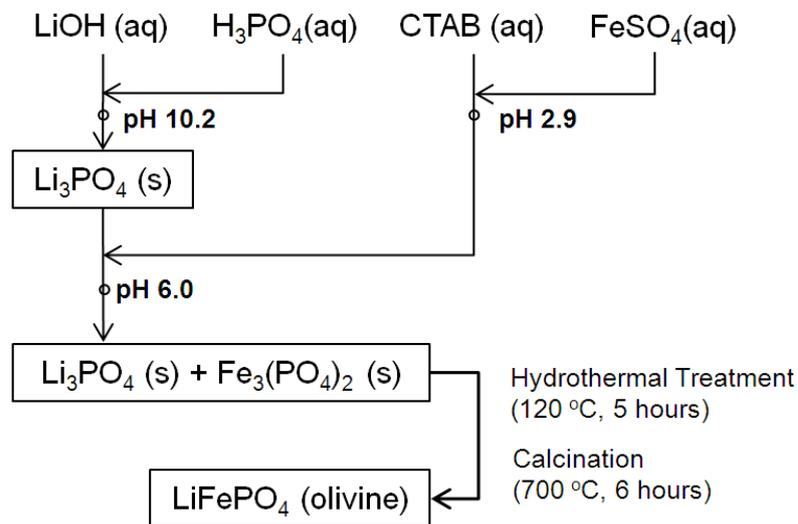
**Figure 4-1: Schematic model over LiFePO<sub>4</sub> production (Myeong-Hee Lee 2010).**
