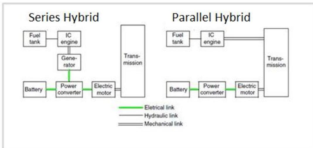
Figure 2-1: Different hybrid vehicle configurations.(Ehsani, Gao et al. 2010)
