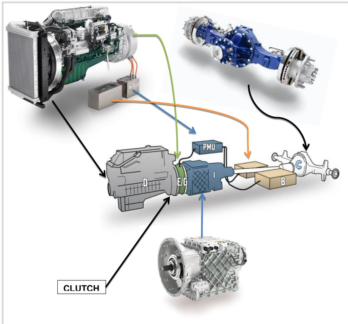
Figure 2-7: Hybrid heavy vehicle drivetrain. (Volvo Trucks 2011)
