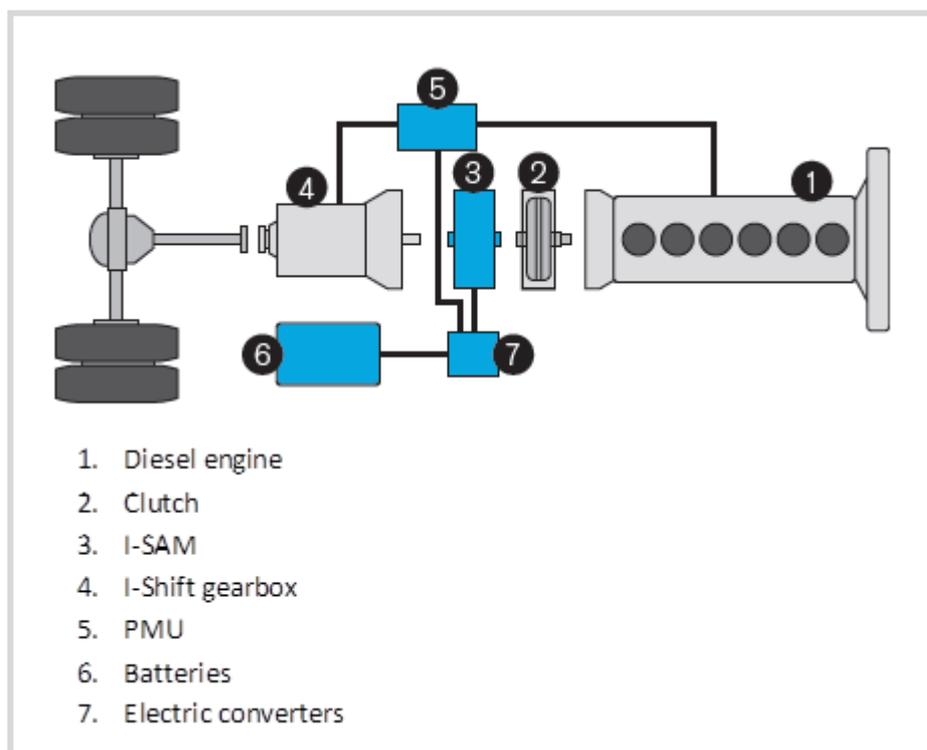
Figure 1-2: Basic overview of the Volvo FE Hybrid drivetrain (Volvo Trucks 2008).
