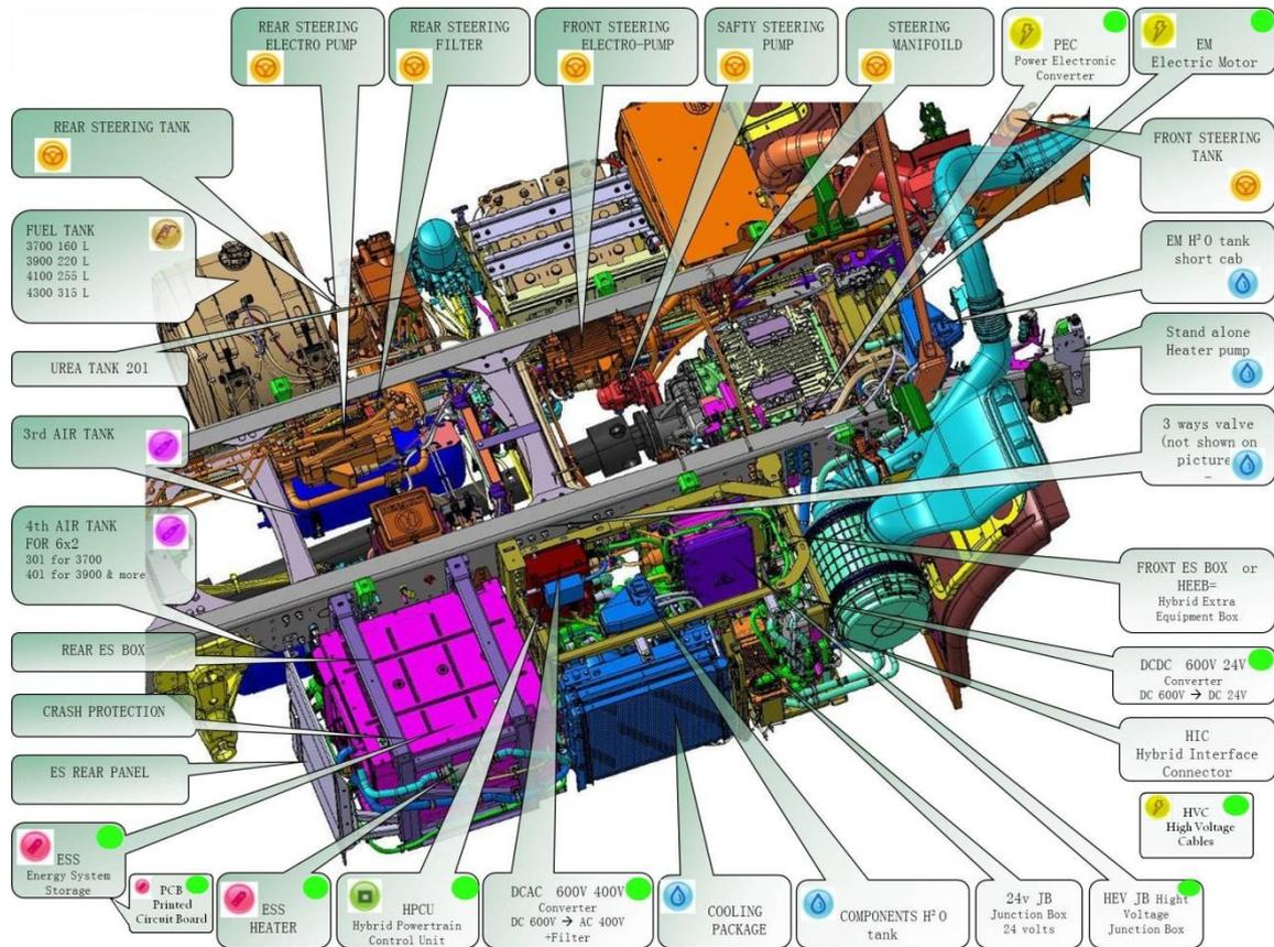
Figure 2-8: A representation of some of the hybrid vehicle components. Boxes with green dots are components included in the study.
