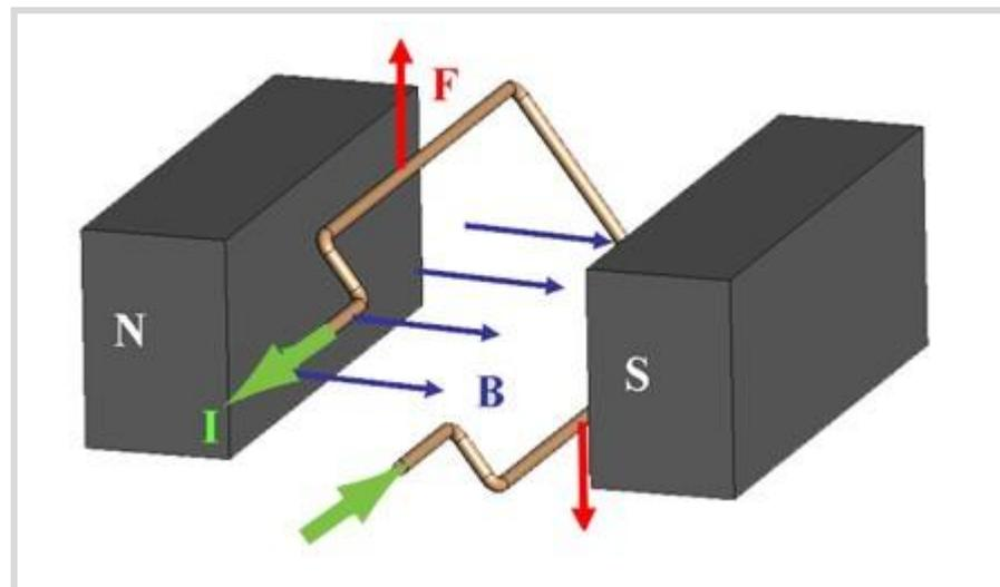
Figure 2-2: Basic DC motor setup. (LIMS 2011)
