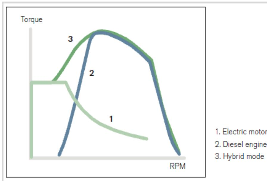
Figure 1-1: Efficiency curve of the different power source configurations (Volvo Trucks 2008).
