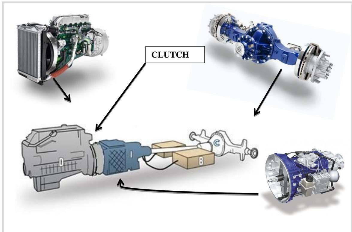
Figure 2-6: Conventional heavy vehicle drivetrain. (Volvo Trucks 2012)
