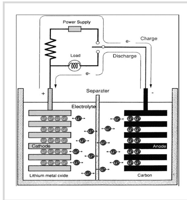
Figure 2-3: Schematic overview of an LFP-battery (Yuan, Liu et al. 2012).
