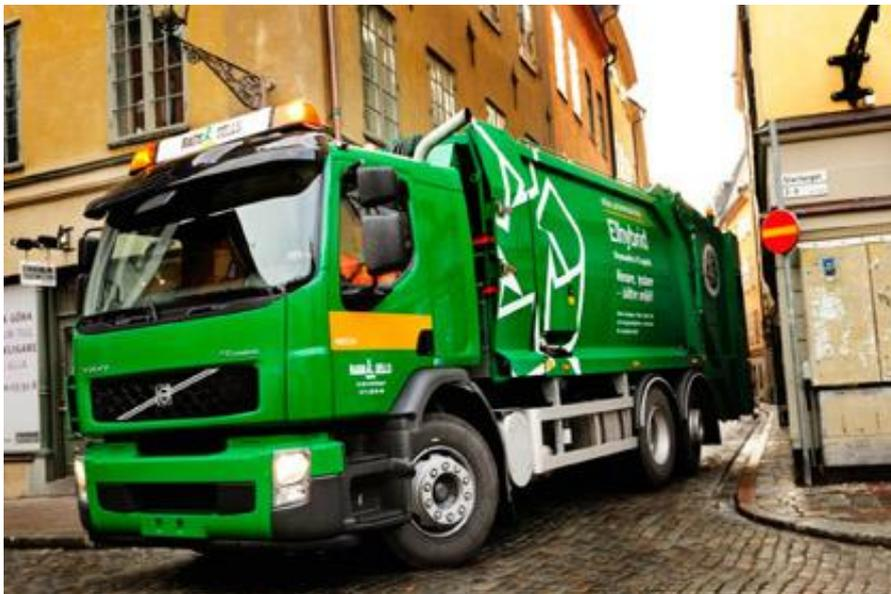
Figure 2-5: Volvo FE Hybrid waste collection vehicle (Volvo Trucks 2012).
