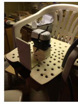
Bilge pump Customized to fit in the bottom of the container to pump urine
