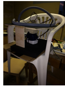
Bilge pump Customized to fit in the bottom of the container to pump urine
