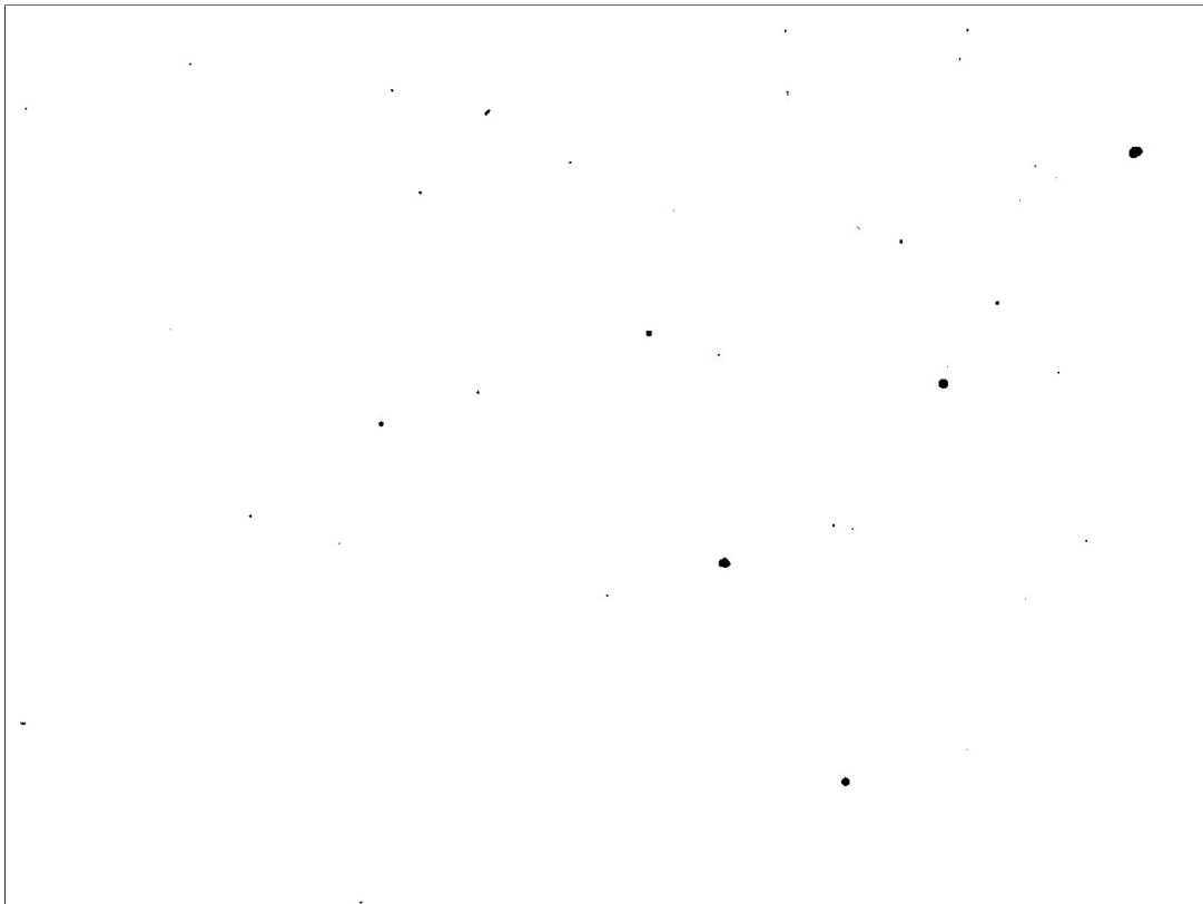
Figure A.2: Scale bar removed and threshold adjusted to only show porosity and not Nitrides. Amount of pores measured, 0,05% in this picture
