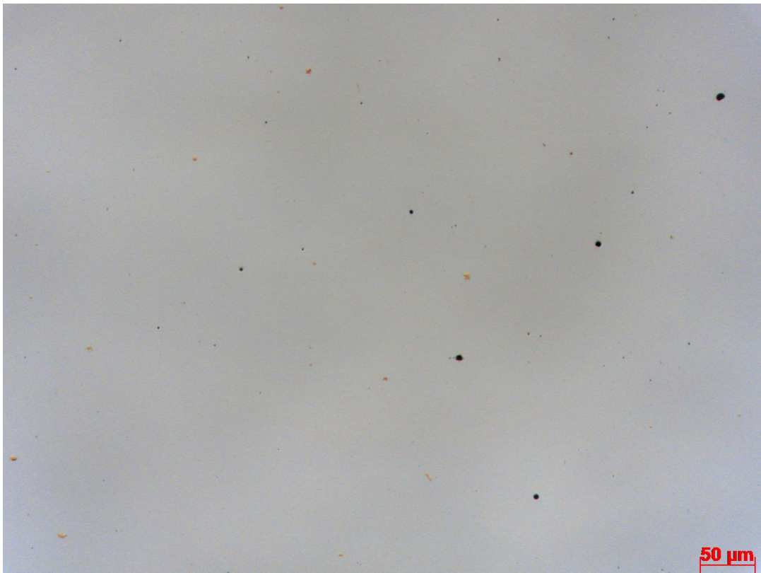
Figure A.1: Picture for porosity measurement. Sample As-built DMLS 10mm cylinder picture 4/15.
