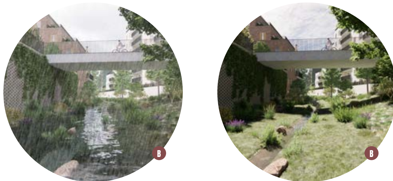
Fig 73. Storm water trench when flooded and in normal state.
