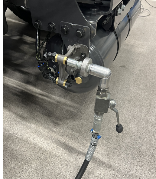
(b) External air supply connection to tank.
