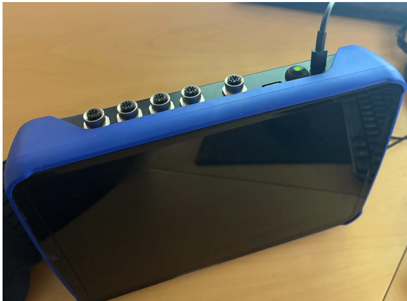
Figure 4.3: Prototype with sensor connections 1–5, power button, and USB ports.
