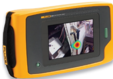
Figure 2.3: Acoustic imager camera of model ii900 [15], where red regions indicate detected acoustic emissions associated with a leak.
