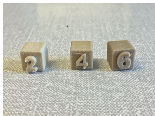
Figure 23 - 3D printed cubes with two, four and six times extruded material.
