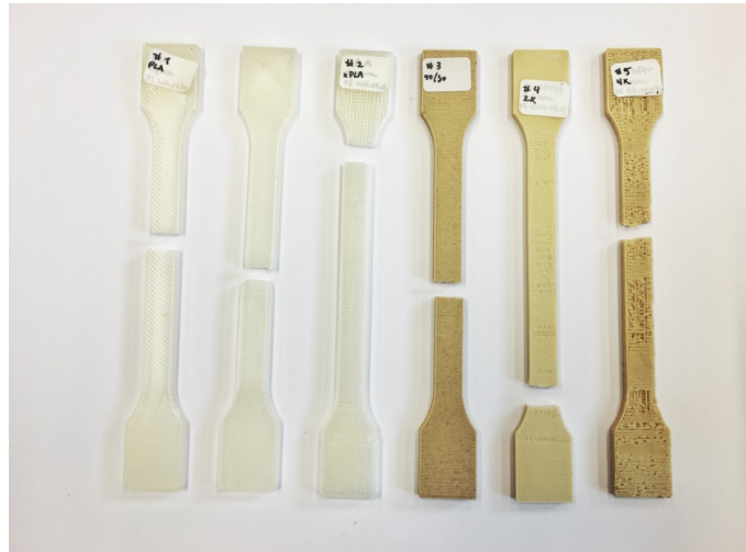
Figure 24 - 3D printed specimens for tensile tests
