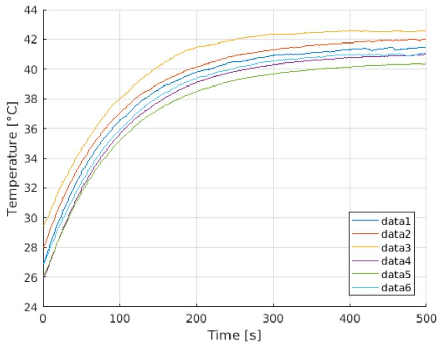
**Figure A.14:** Bundle test – multiple conductive cables supplied with 24 [V] and 25 [A].
