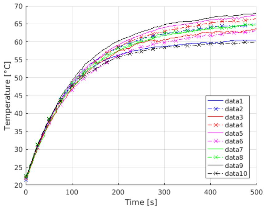
**Figure A.9:** Long cable test supplied with 48 [V] and 25 [A].
