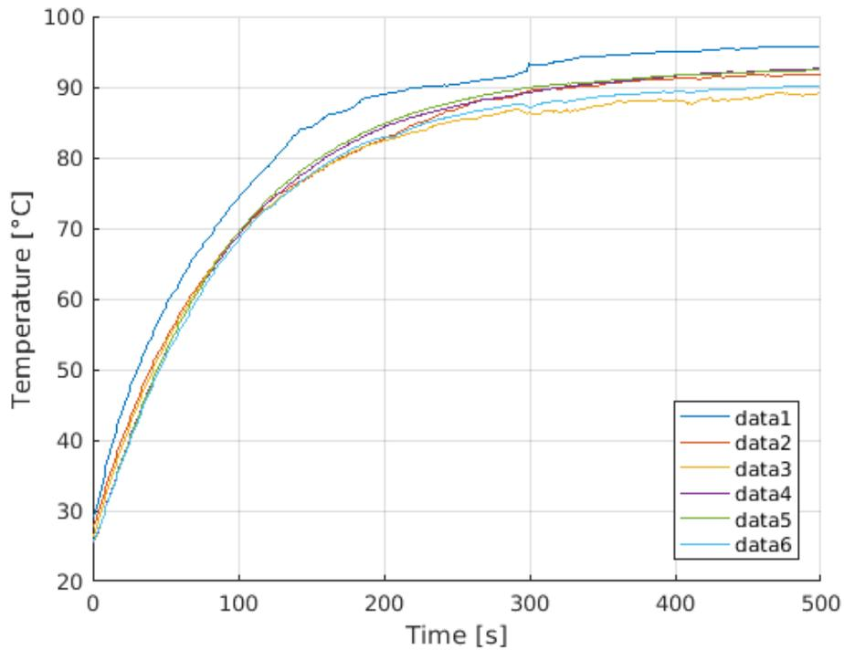
**Figure 4.16:** Bundle test – multiple conductive cables supplied with 24 [V] and 50 [A].
