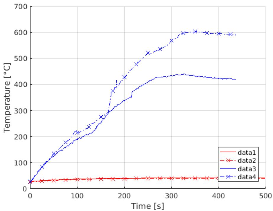
**Figure 4.21:** Mixed bundle test with multiple conductive cables supplied with 24 [V] and 25 [A].
