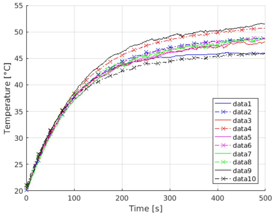
Figure 4.8: Long cable test supplied with 24 [V] and 20 [A].
