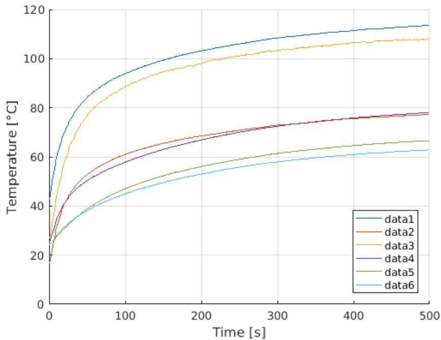
**Figure A.12:** Bundle test – single conductive cable supplied with 48 [V] and 25 [A].
