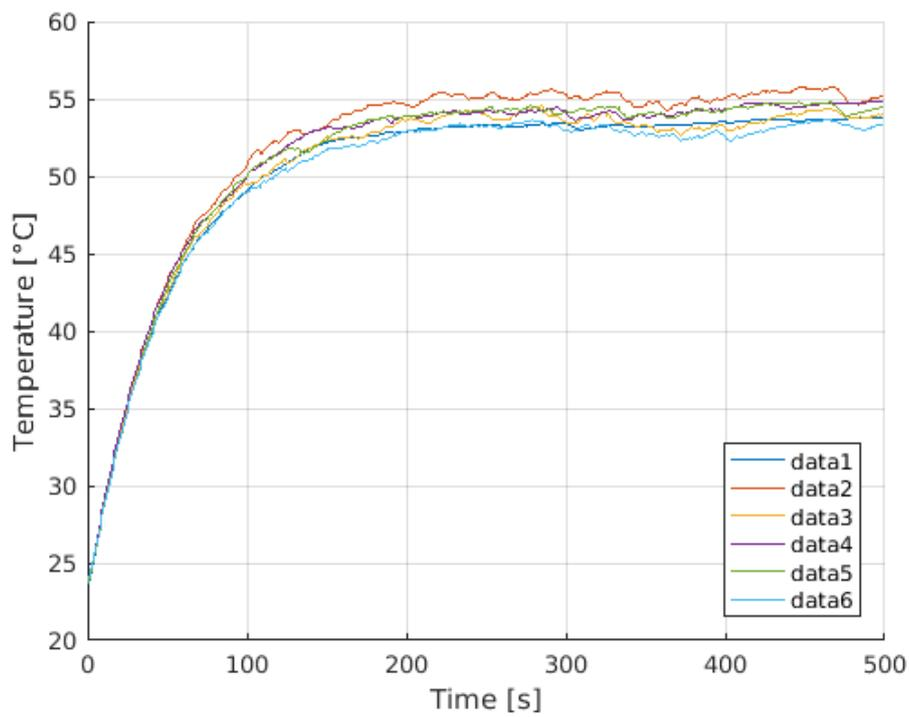
**Figure 4.4:** Single conductive cable supplied with with 48 [V] and 20 [A].
