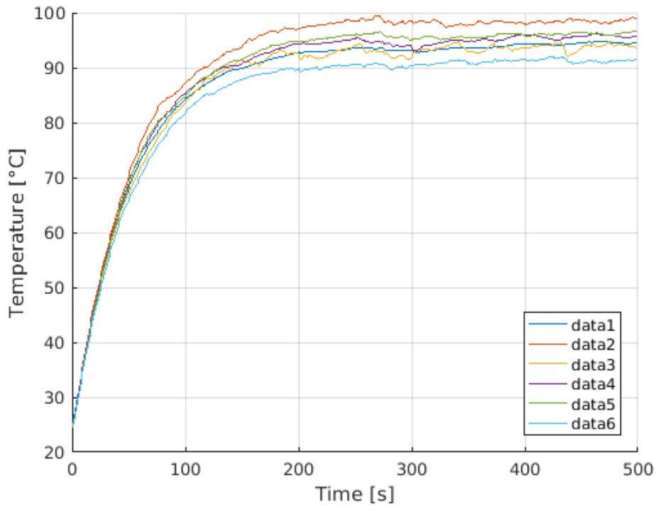
**Figure 4.5:** Single conductive cable supplied with with 24 [V] and 30 [A].
