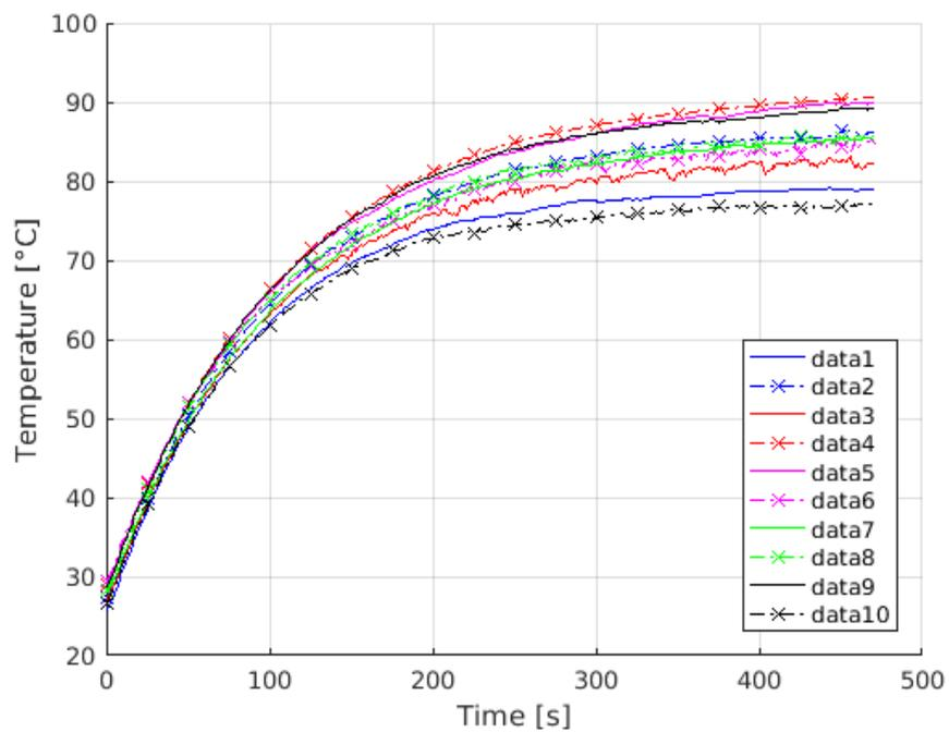
**Figure A.10:** Long cable test supplied with 48 [V] and 30 [A].
