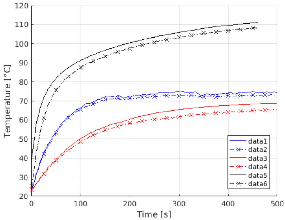
**Figure 4.20:** Mixed single conducting cables test supplied with 24 [V] and 25 [A].
