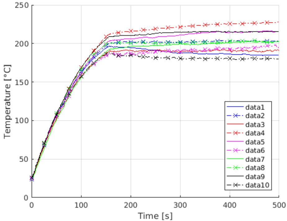
Figure 4.10: Long cable test supplied with 24 [V] and 55 [A].
