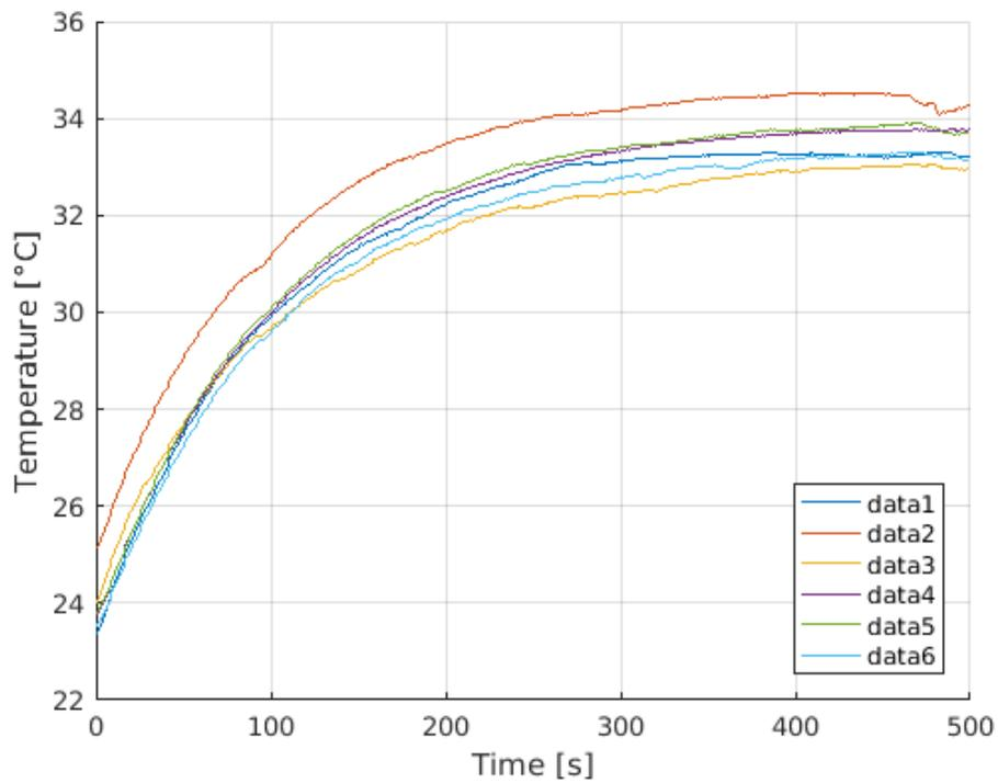
**Figure 4.13:** Bundle test – multiple conductive cables supplied with 24 [V] and 20 [A].
