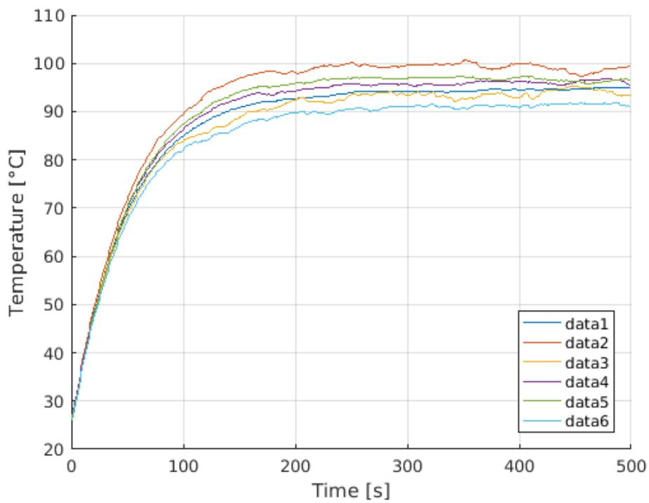
**Figure 4.6:** Single conductive cable supplied with with 48 [V] and 30 [A].
