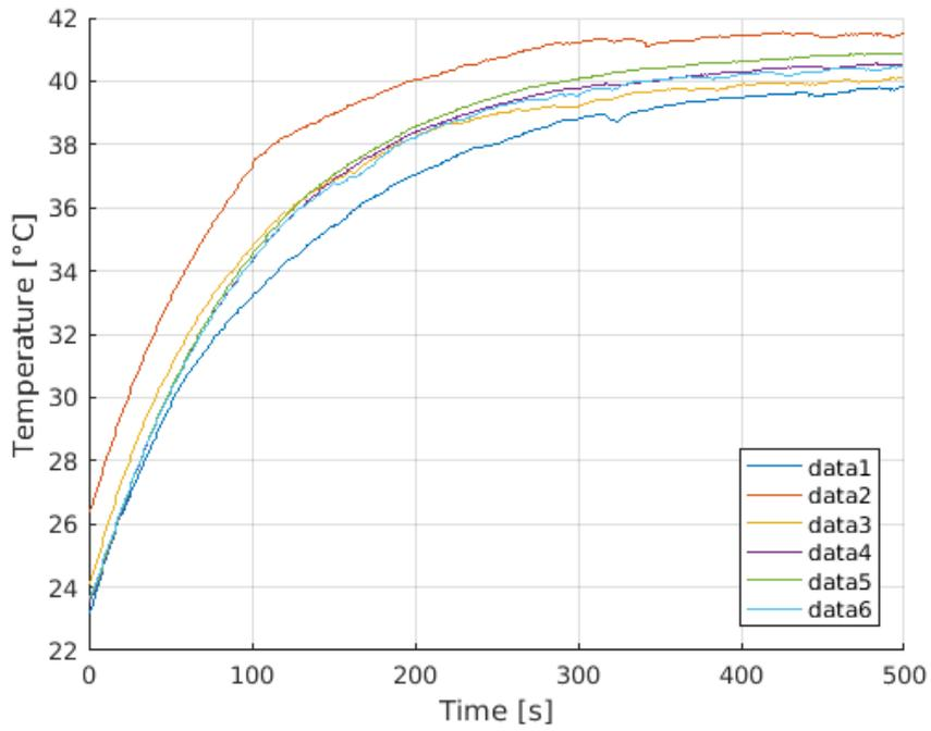
**Figure A.15:** Bundle test – multiple conductive cables supplied with 48 [V] and 25 [A].
