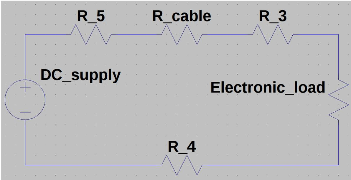
**Figure 4.2:** Picture of the electrical circuit used for the testing rig complete with each resistance demonstrating which cable was used.
