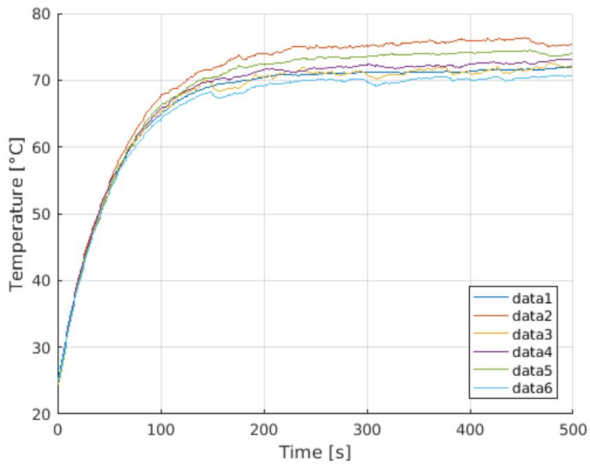
**Figure A.6:** Single conductive cable supplied with with 48 [V] and 25 [A].
