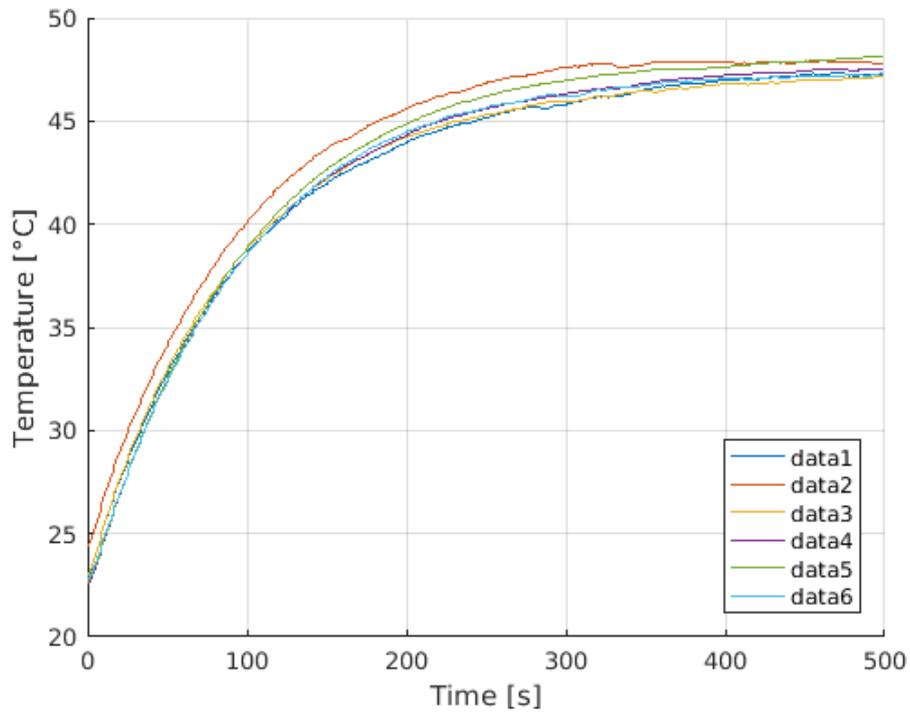
**Figure 4.14:** Bundle test – multiple conductive cables supplied with 24 [V] and 30 [A].
