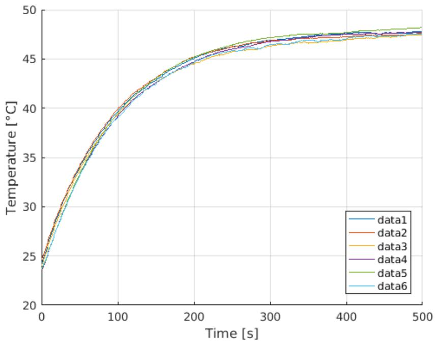
**Figure A.16:** Bundle test – multiple conductive cables supplied with 48 [V] and 30 [A].
