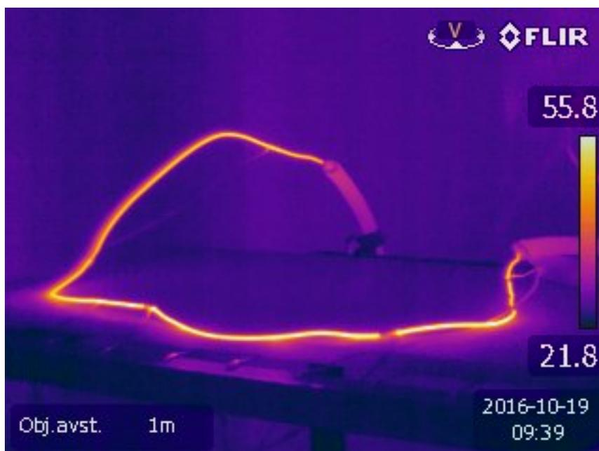
**Figure A.2:** IR picture of single conductive cable supplied with with 48 [V] and 25 [A].
