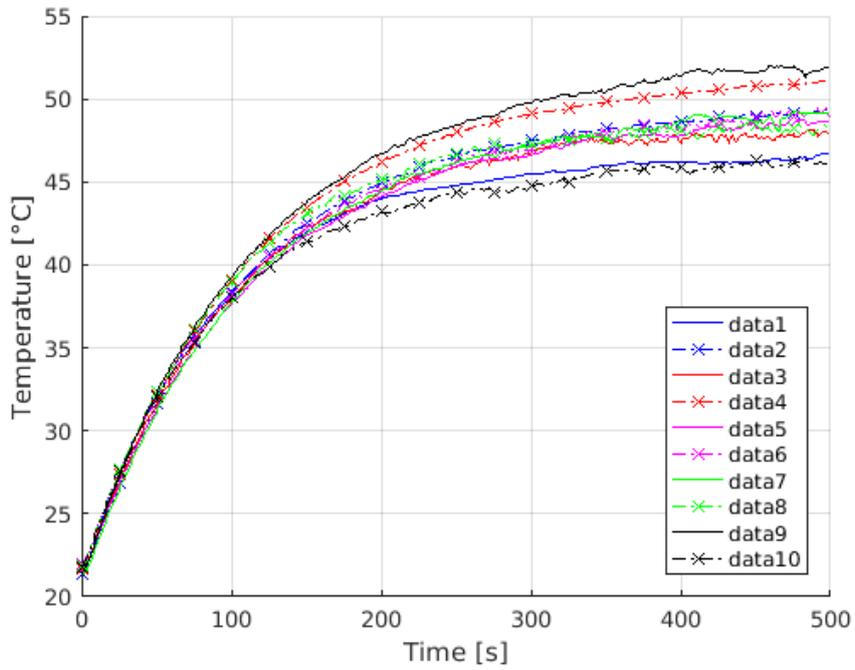
Figure A.7: Long cable test supplied with 48 [V] and 20 [A].
