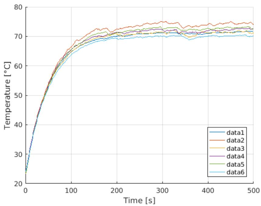
**Figure A.5:** Single conductive cable supplied with with 24 [V] and 25 [A].
