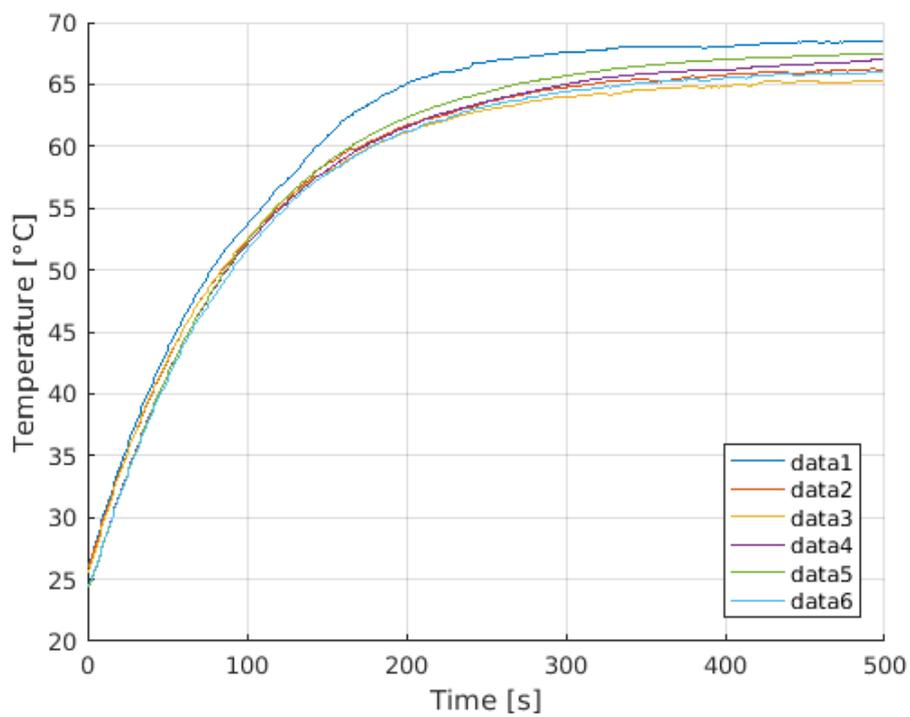
**Figure 4.15:** Bundle test – multiple conductive cables supplied with 24 [V] and 40 [A].
