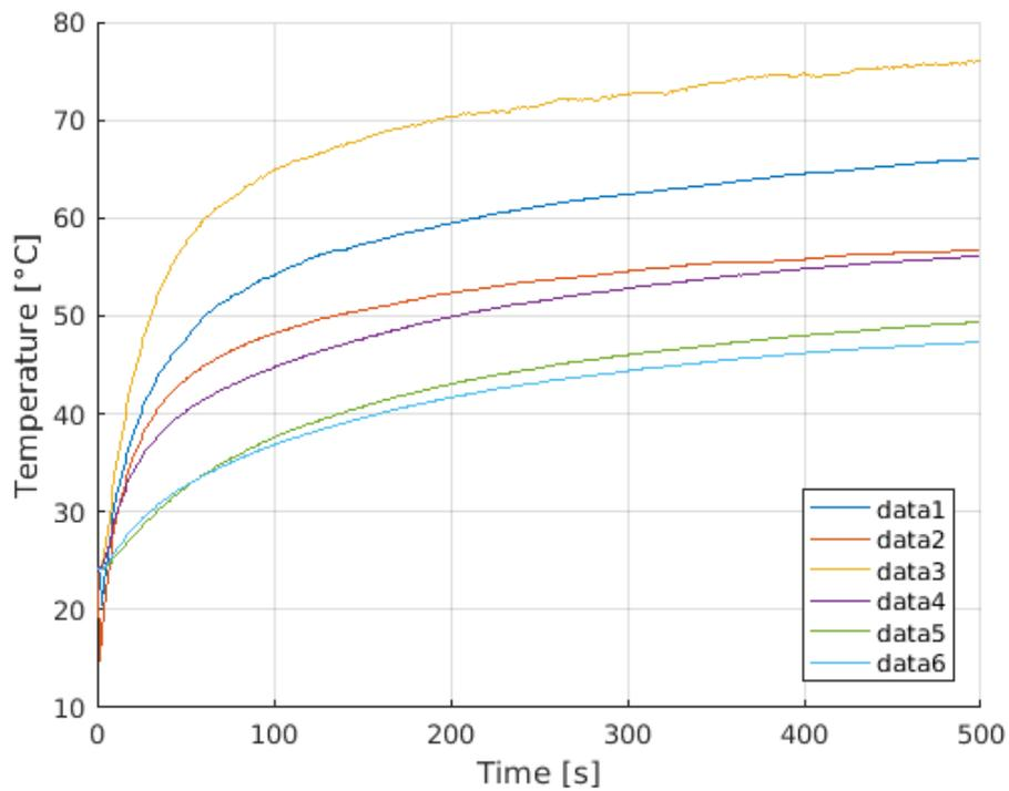
**Figure 4.11:** Bundle test – single conductive cable supplied with 24 [V] and 20 [A].
