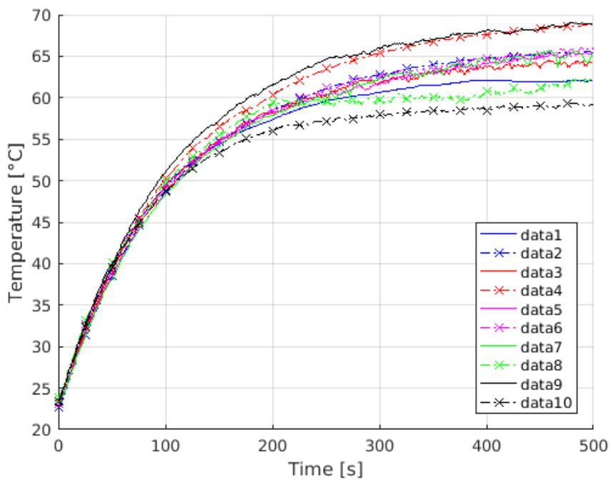
Figure A.8: Long cable test supplied with 24 [V] and 25 [A].
