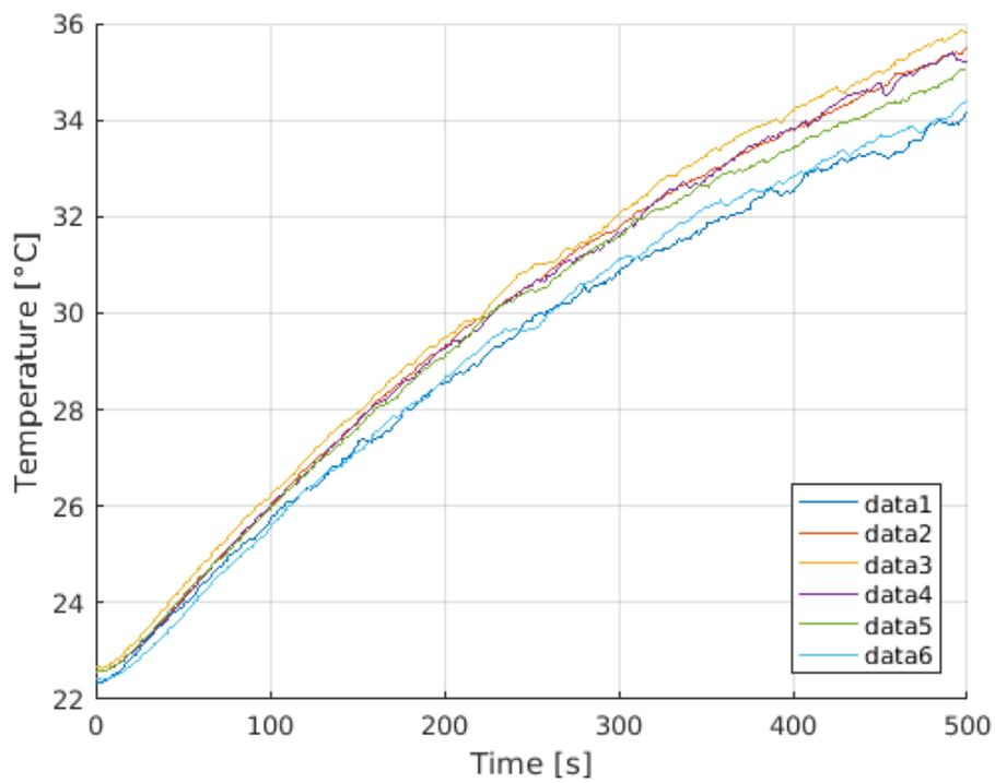
**Figure 4.19:** Power cable supplied with 24 [V] and 105 [A].
