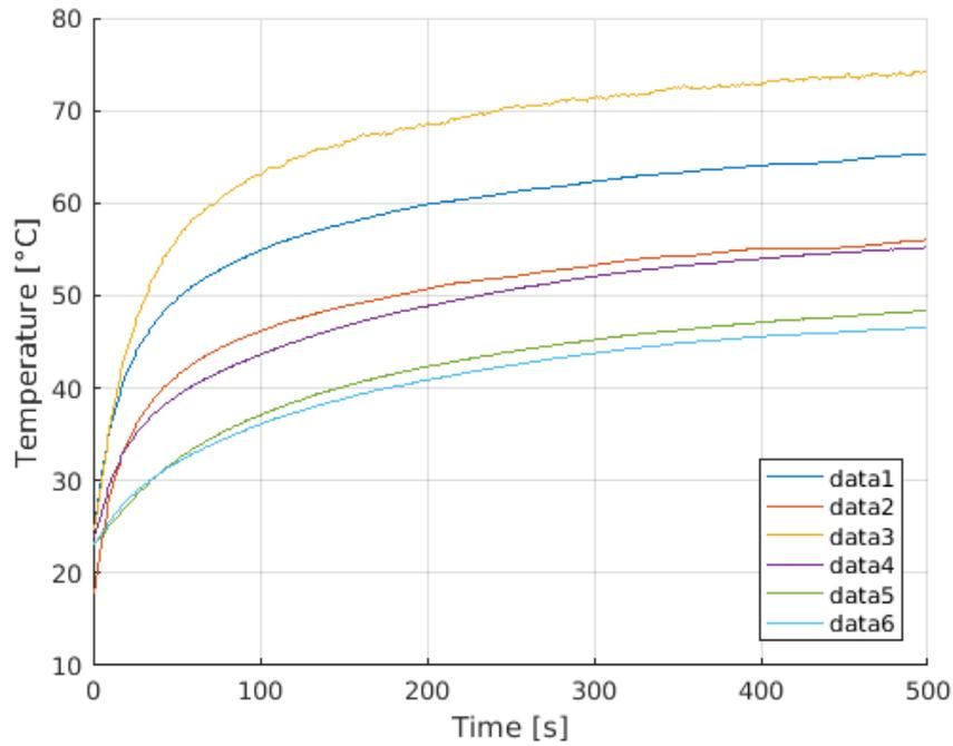
**Figure A.11:** Bundle test – single conductive cable supplied with 48 [V] and 20 [A].
