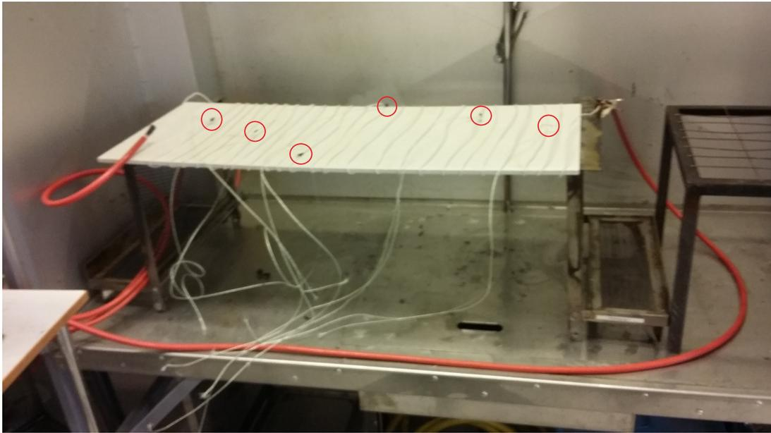
**Figure 4.7:** Test rig of the long cable test with thermocouples encircled.
