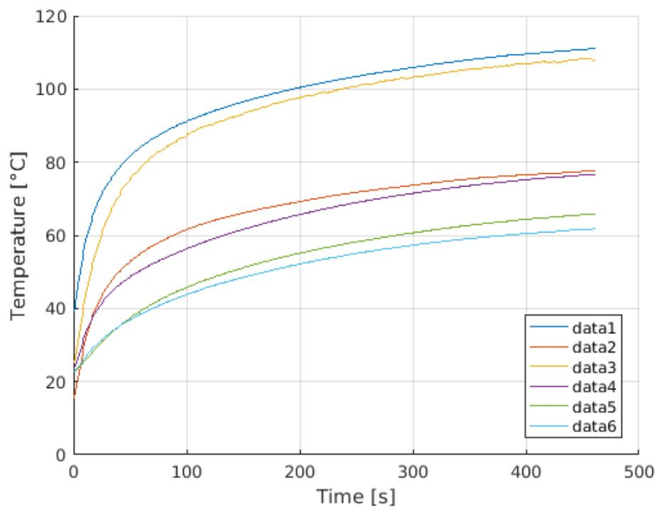
**Figure 4.12:** Bundle test – single conductive cable supplied with 24 [V] and 25 [A].
