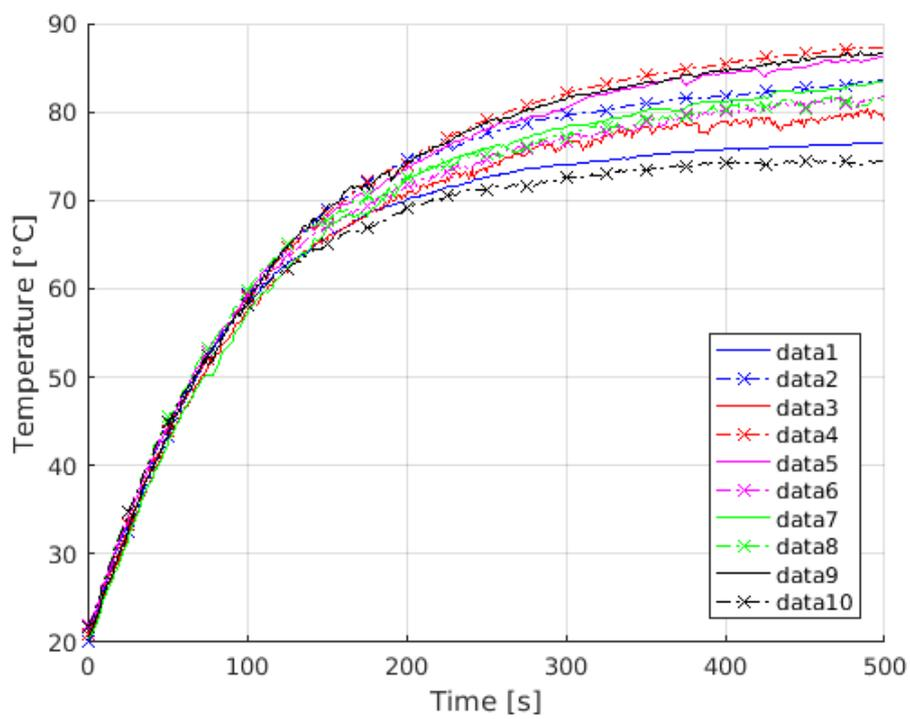
Figure 4.9: Long cable test supplied with 24 [V] and 30 [A].
