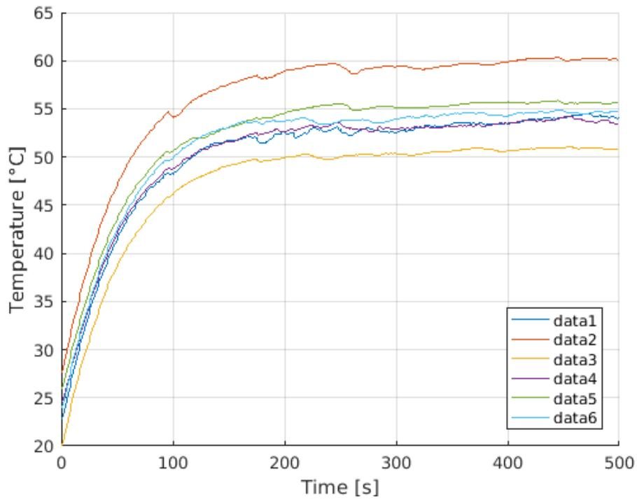
**Figure 4.3:** Single conductive cable supplied with with 24 [V] and 20 [A].
