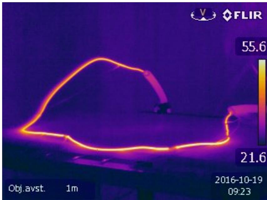
**Figure A.1:** IR picture of single conductive cable supplied with with 24 [V] and 25 [A].
