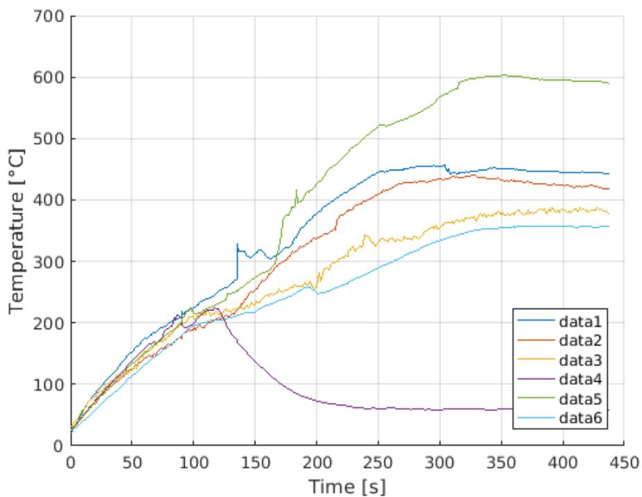
**Figure 4.17:** Bundle test – multiple conductive cables supplied with 24 [V] and 100 [A] with a car battery.
