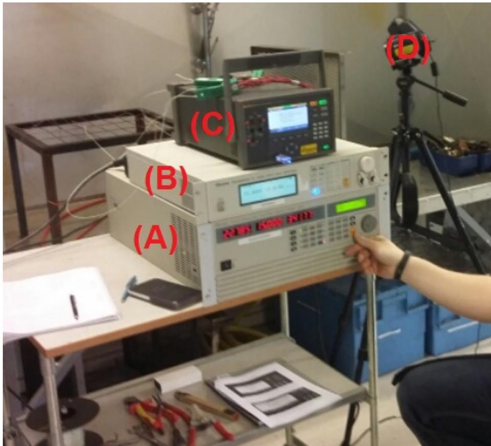
**Figure 4.1:** Picture of the test rig in use, in the picture the (A) electric load, (B) electric source, (C) data acquisition machine and the (D) infrared camera.
