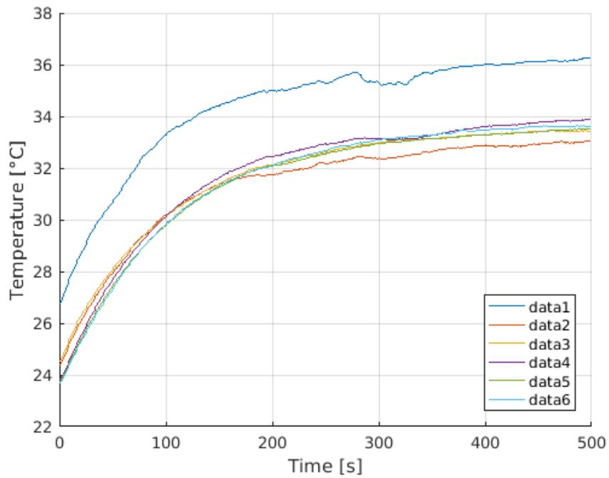
**Figure A.13:** Bundle test – multiple conductive cables supplied with 48 [V] and 20 [A].
