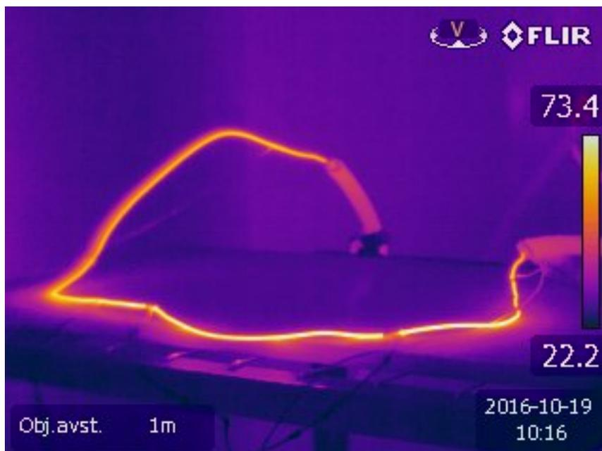
**Figure A.4:** IR picture of single conductive cable supplied with with 48 [V] and 30 [A].
