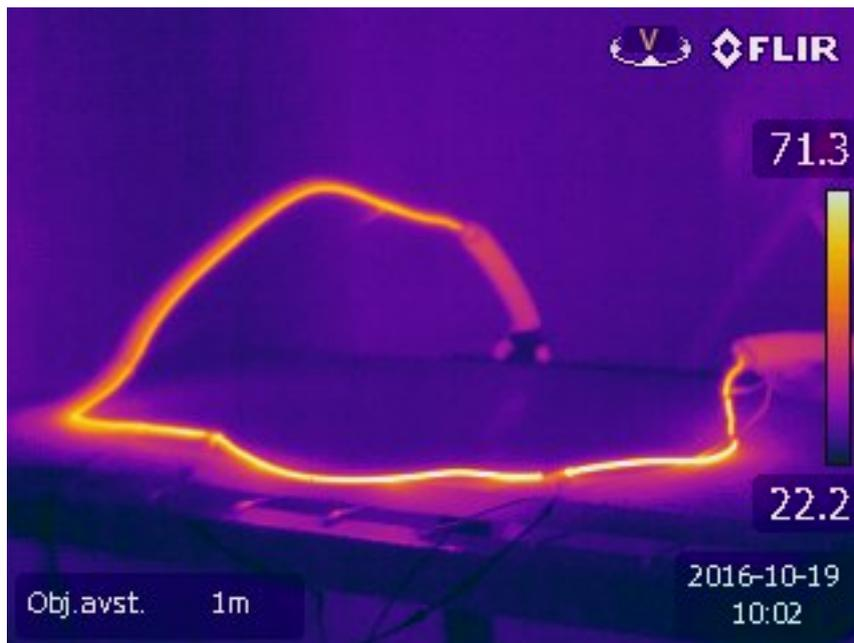
**Figure A.3:** IR picture of single conductive cable supplied with with 24 [V] and 30 [A].
