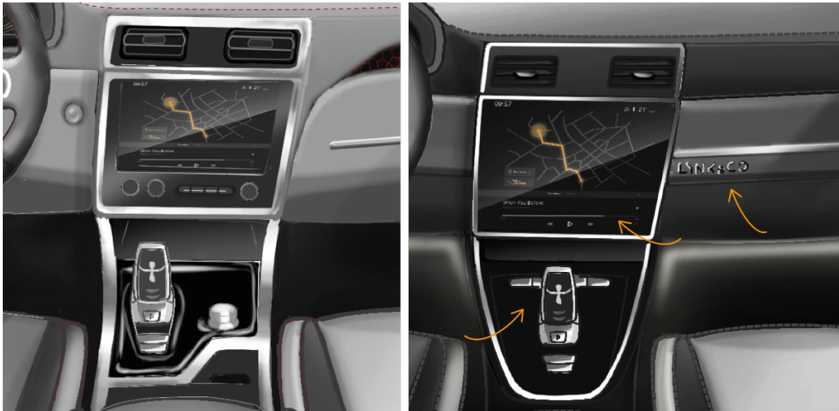
Figure 20. Comparison original (left) with re-design (right) infotainmentsystem and gearshift area
