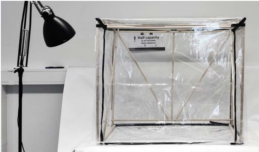
Figure 73: Homemade laminar for experiment setup
