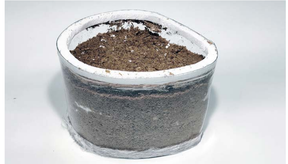
Figure 58: Casting the prototype - Composite: Oyster fungi inoculated into straw and corn seed
