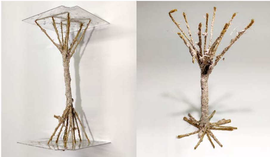
Figure 84: Lion's mane composite applied on twisted rope of tower structure
