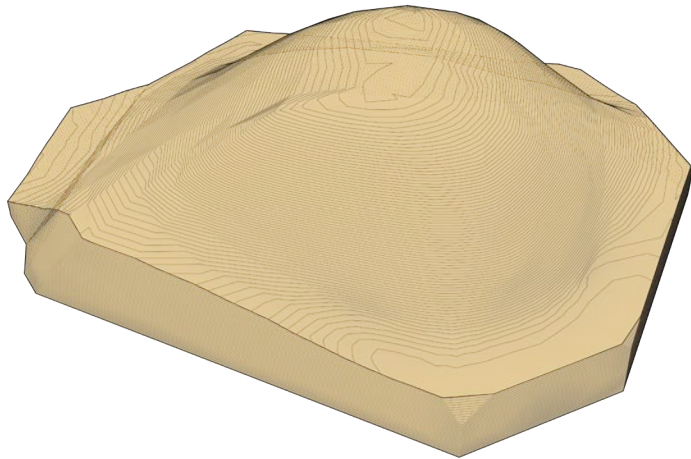
Figure 35: 3D model of a mould sample for 3D printing in scale of 1 : 10 (15x15x5 cm)
