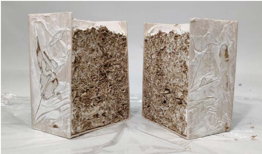
Figure 77: Oyster composite - The sample with 10 cm thickness cut in half
