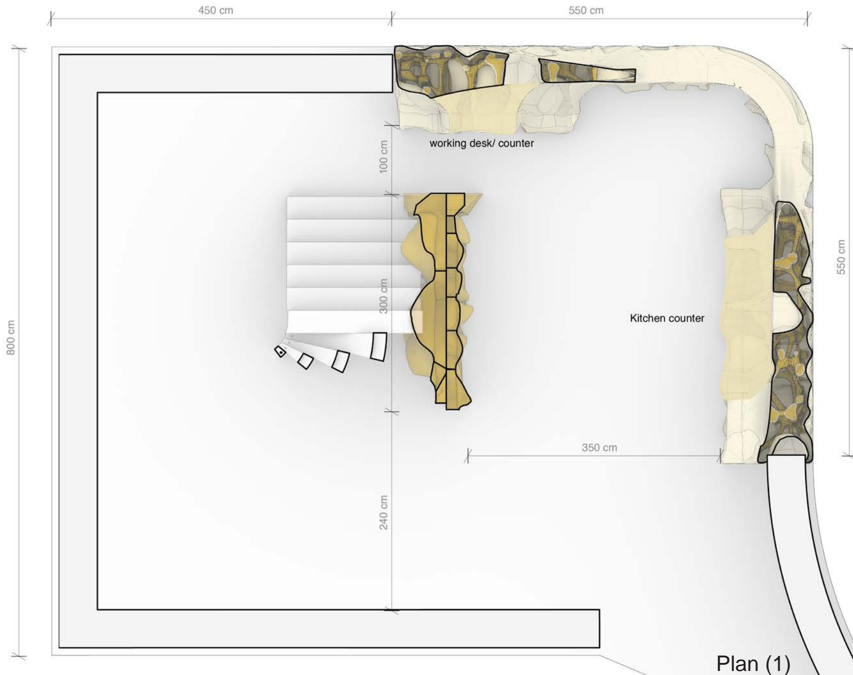
Figure 24: New plan layout of C-Hive project - Scale 1 : 50
