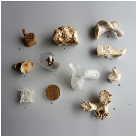
Figure 61: 3D print iterative testing of Mycelium chair (Pallister, 2014)
