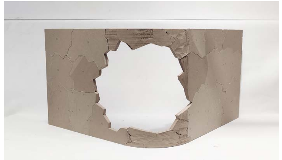
Figure 40: Assembled exterior moulds - Scale 1 : 10
