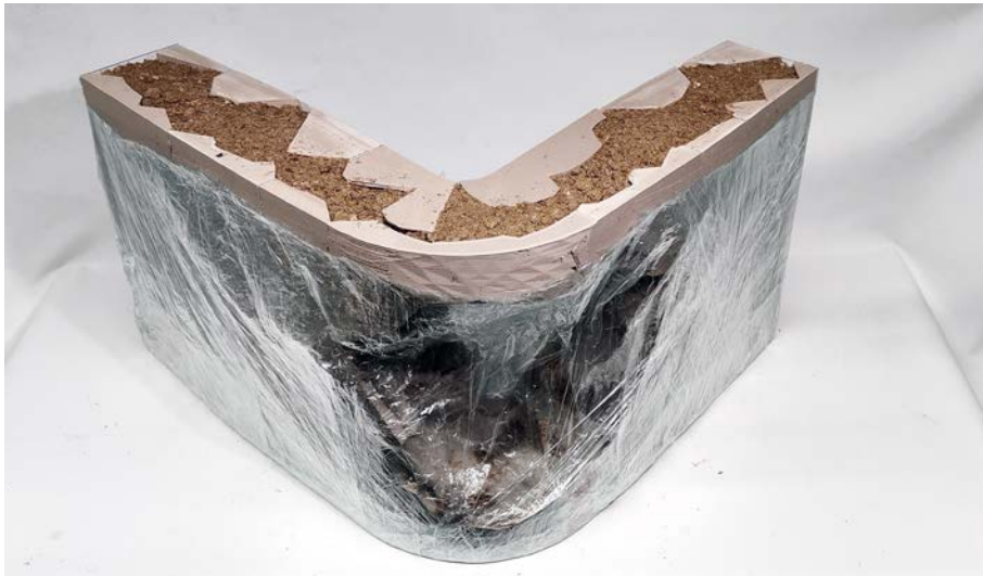
Figure 43: Casting the prototype - Composite: Oyster fungi inoculated into straw and corn seed
