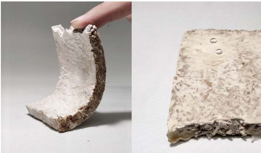
Figure 78: Left: Flexibility of the sample with 1 cm thickness - Right: Testing hydrophobicity
