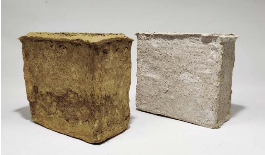
Figure 75: Single-use moulds made of mashed paper
