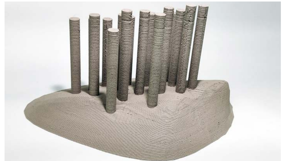
Figure 59: 3D printed mould with light wooden PLA - Scale 1 : 2
