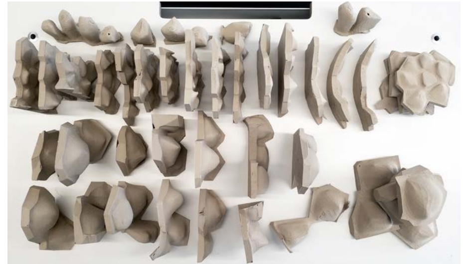
Figure 36: 46 pieces of 3D printed moulds with light wooden PLA - Scale 1 : 10
