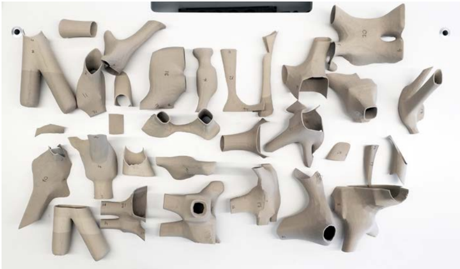
Figure 50: 25 pieces of 3D printed cavity element with light wooden PLA - Scale 1 : 2
