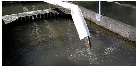
Figure 13: A fish exits the Salmon Cannon TM (Whooshh innovations (2018b)).
