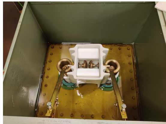
(b) The container with the volume filler mounted in the dielectric strength tester.
