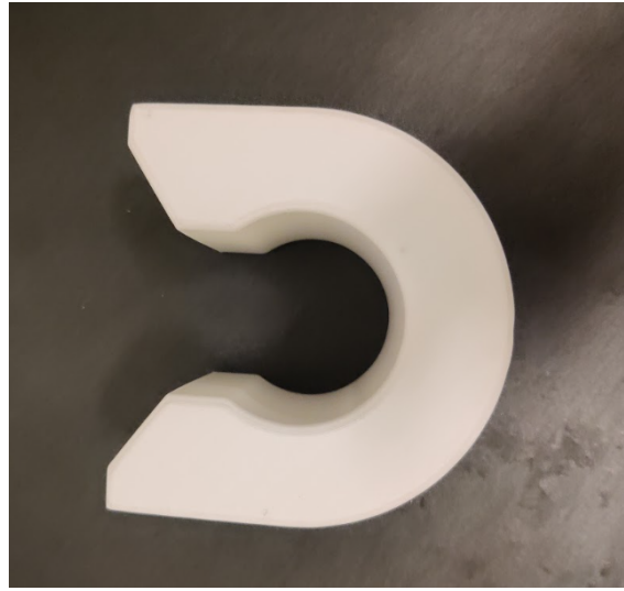
Figure 3.2: Volume filler made out of polypropylene.
