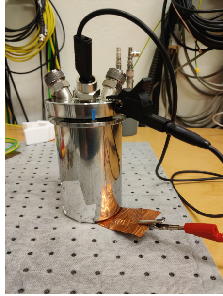
(b) Connection setup to Tettex 2093a.
