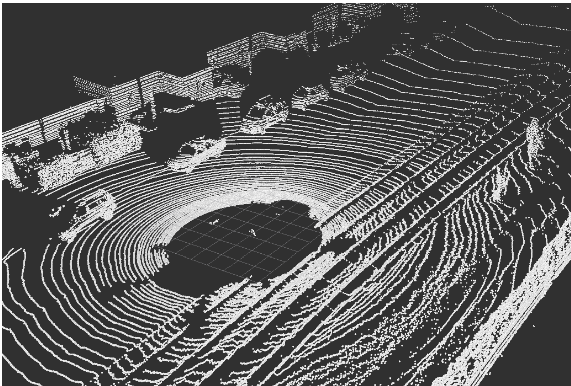
Figure 4.1: A LiDAR frame's pointcloud2 displayed in RVIZ.
