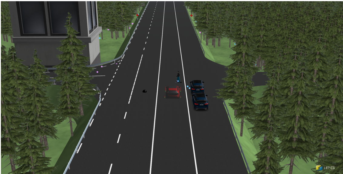
Figure 3.10: Screenshot from IPG CarMaker Showing Detection Points Created Using RSI Radar.
