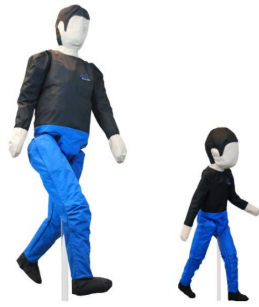
Figure 3.5: Euro NCAP Pedestrian Dummy Targets (Adult on the left and Child on the right)
