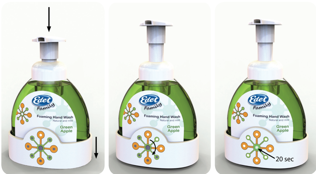
Figure 29. From the left: The pump is pushed and the timer is activated. The lights turn on clockwise with a 2.5 second interval. The sequence ends with a green light in the middle on the 20th second..
