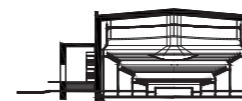
1:500 A section of the lobby and concert hall, with the position of the lowered ceiling dashed.
