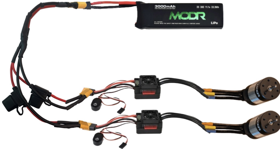
Figure 3.5: Physical connections of battery, adapter, and ESC to test setup.
