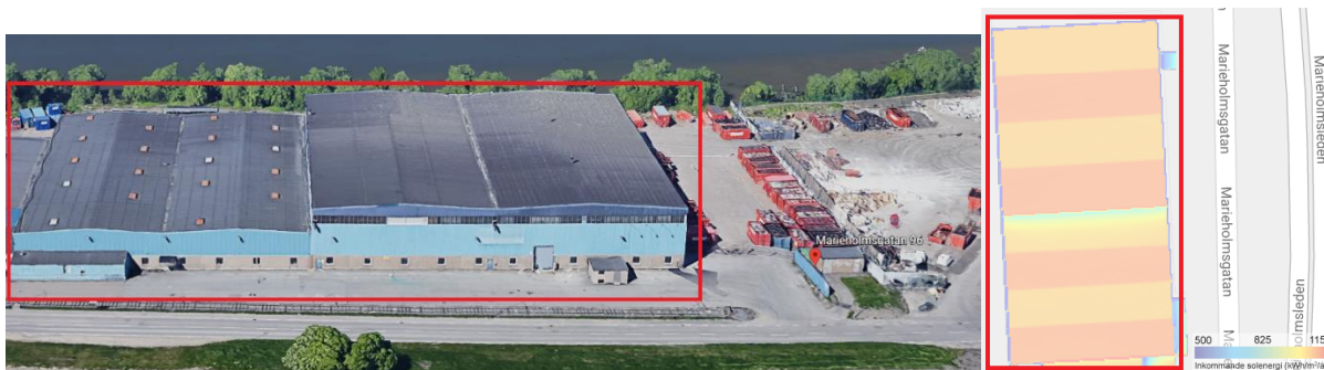
Figure 12: Rödingen balling station rooftop and cross-sectional view (left). Source of image: (Google Earth, n.d.-b) Solar irradiation potential for the rooftop at Rödingen (right). Source of image: (Göteborg Energi, 2020b)
