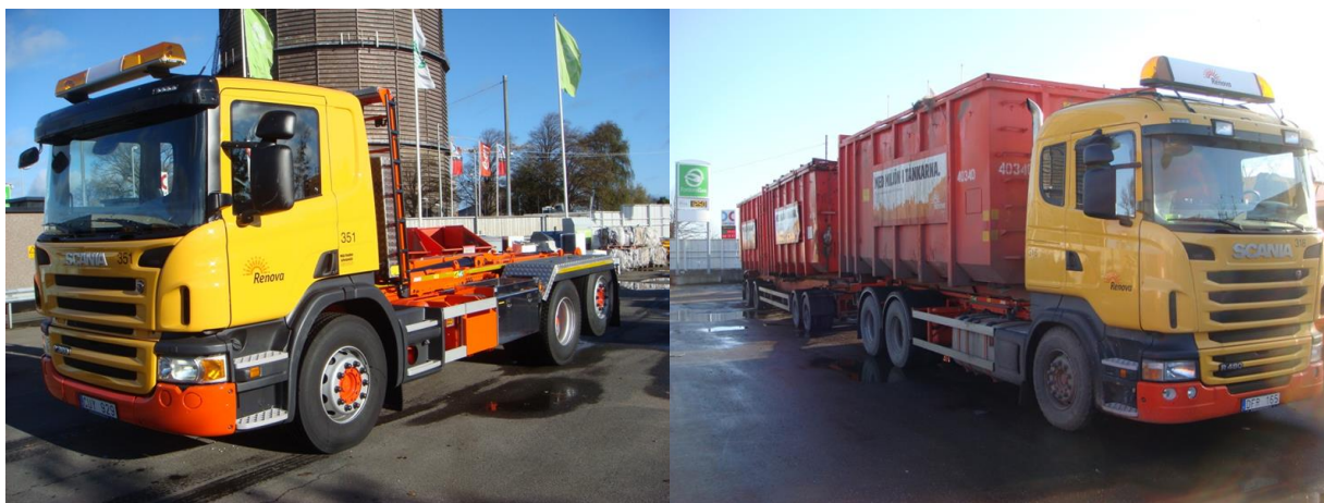
Figure 51: Hook lift truck unloaded and loaded along with loaded trailer (H. Zackrisson personal communication, April 27, 2020).
