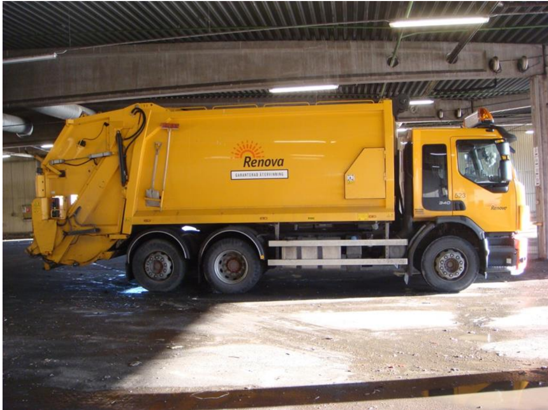
Figure 3: Refuse collector truck side view, with a 2-slot refuse collector. The fuel cell driven truck can be assumed to look approximately the same (H. Zackrisson personal communication, April 27, 2020).
