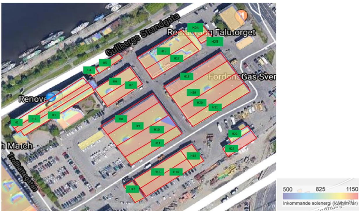
Figure 22: Buildings found at Renova's headquarter and their expected solar irradiation energies. Source of image: (Göteborg Energi, 2020a)
