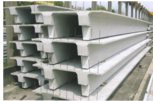
Figure 2.7: TT slab. Photo credit: Elematic.
