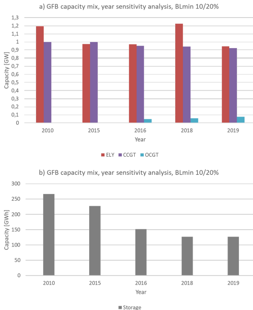
Figure 4.9: Capacity mix of the GFB components with BLmin 10/20% at 5 different year scenarios and a hydrogen price of 4 €/kg. (a. Electrolyzer, CCGT, and OCGT capacities. b. Storage capacity)
