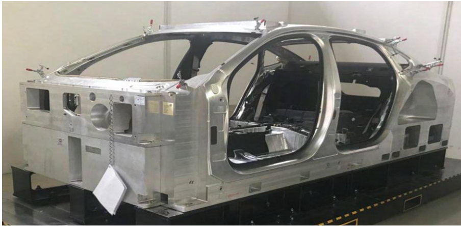
Figure 2.2: One of Polestar’s nominal bucks. The photo has been brought from internal sources (Polestar, 2025).
