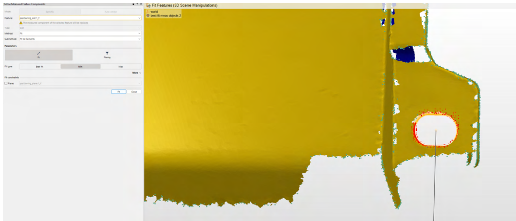
Figure E.14: The slot marked with the window open for doing a best fit to create the slot feature.
