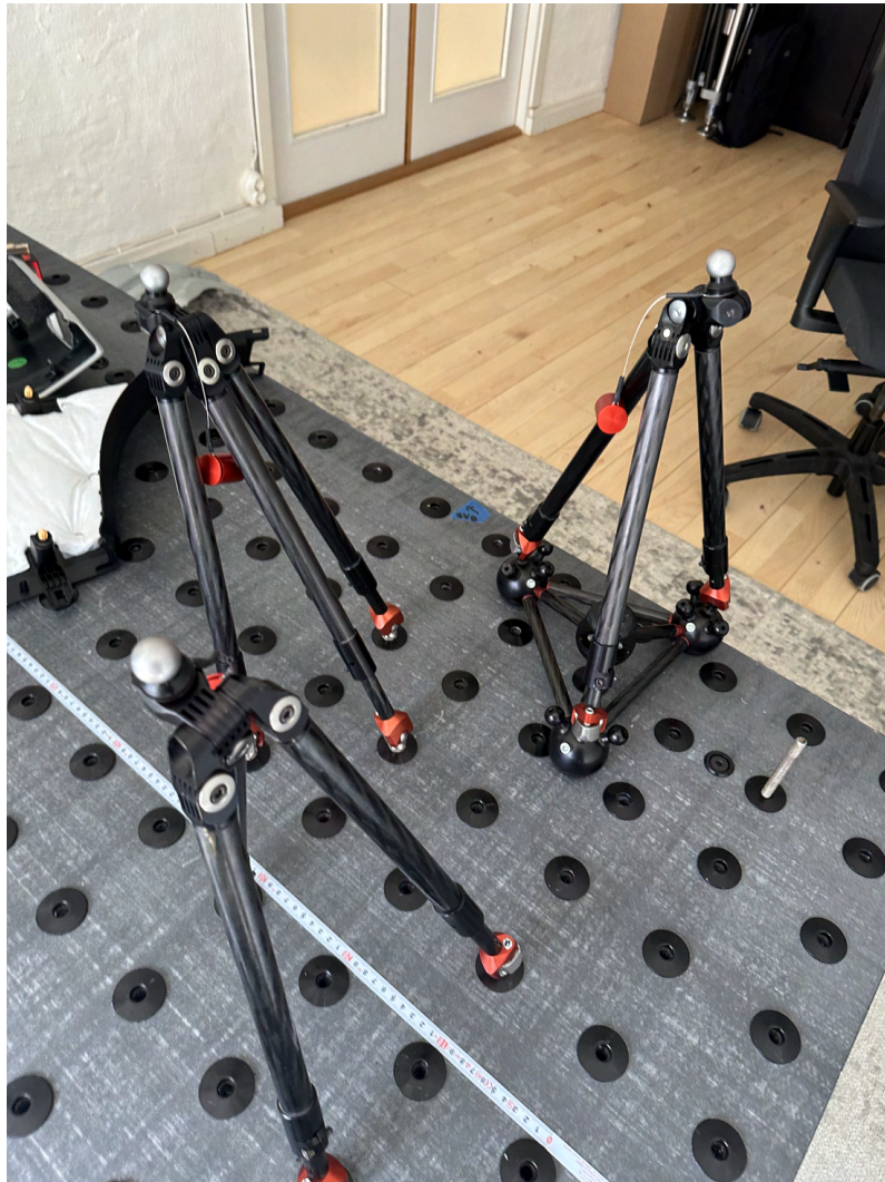
Figure E.4: The finalized sphere setup for the lower part used in the case study.
