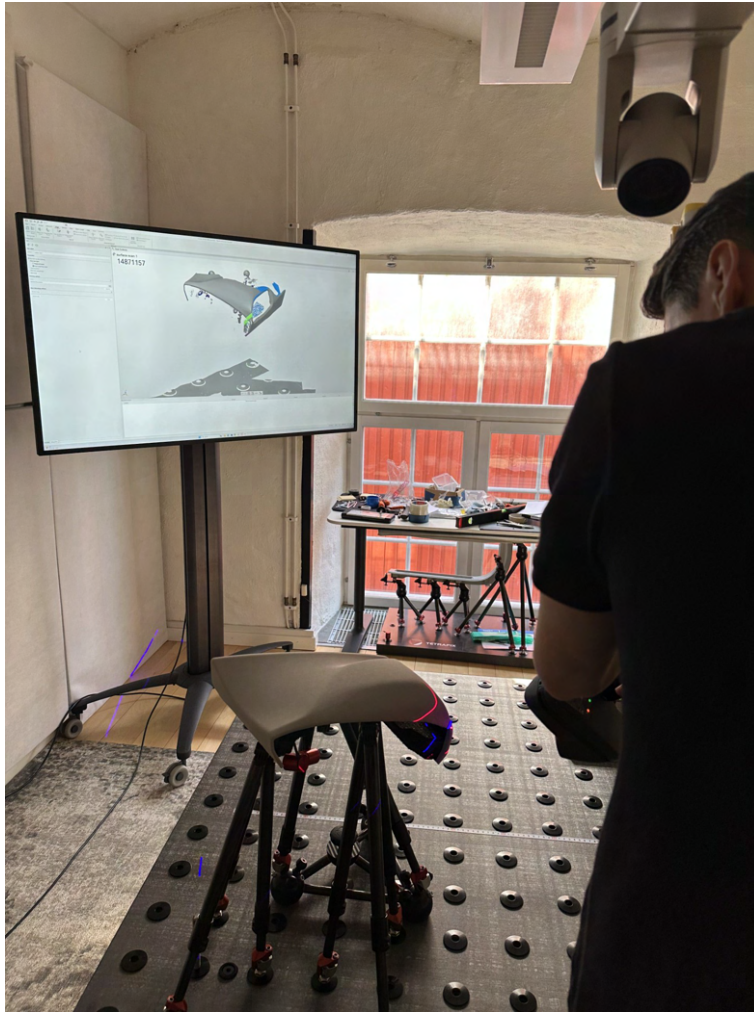
Figure E.8: The scanning process during the case study. Note that in this case it is part Intermediate, which is the other part used during the case study. The text and other figures refers to the other part Lower.
