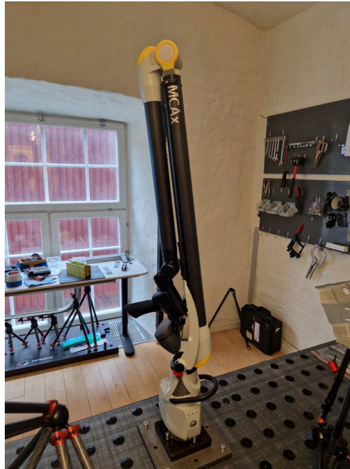
Figure 2.10: Scanner-mounted articulated arm CMM.
