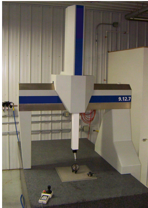
Figure 2.9: 3-axis probe-mounted bridge-type CMM (Wikimedia, 2009).
