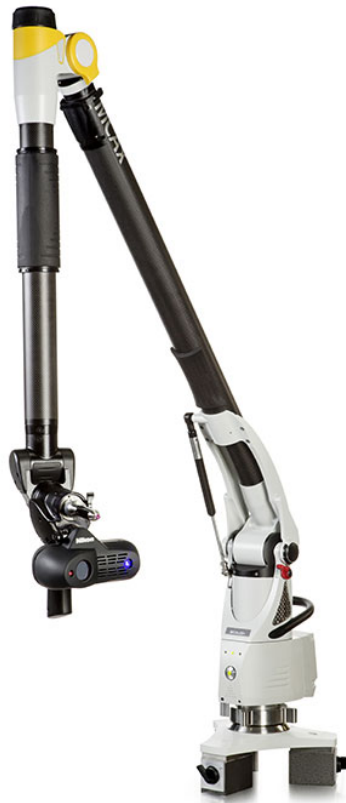
Figure E.2: The articulated CMM arm and laser scanner from Nikon Metrology used during the scanning process.
