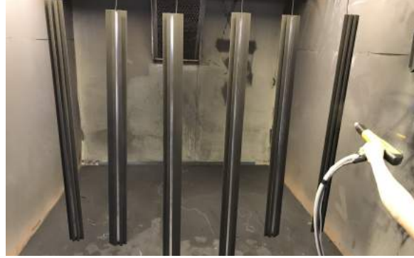
Figure 8.2: Powder coating of the Outer and Inner Profiles.
