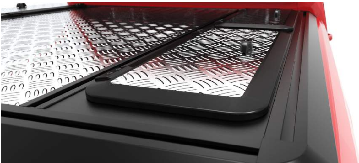
Figure 7.5: Side Opening mounted to the Aluminium Frame.
