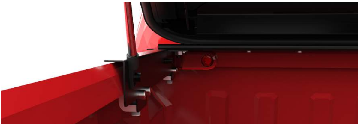
Figure 7.10: Illustration of the clamping solution.
