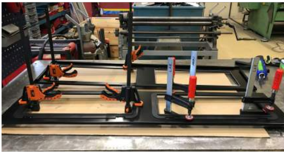
Figure 8.3: Bottom Hatch Frame glued to Sidesheets.
