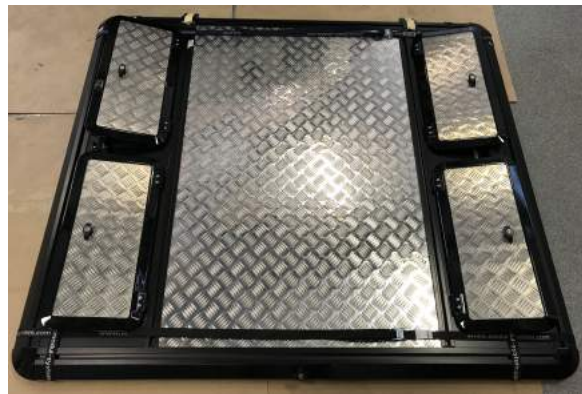
Figure 8.6: Strapped after gluing.
