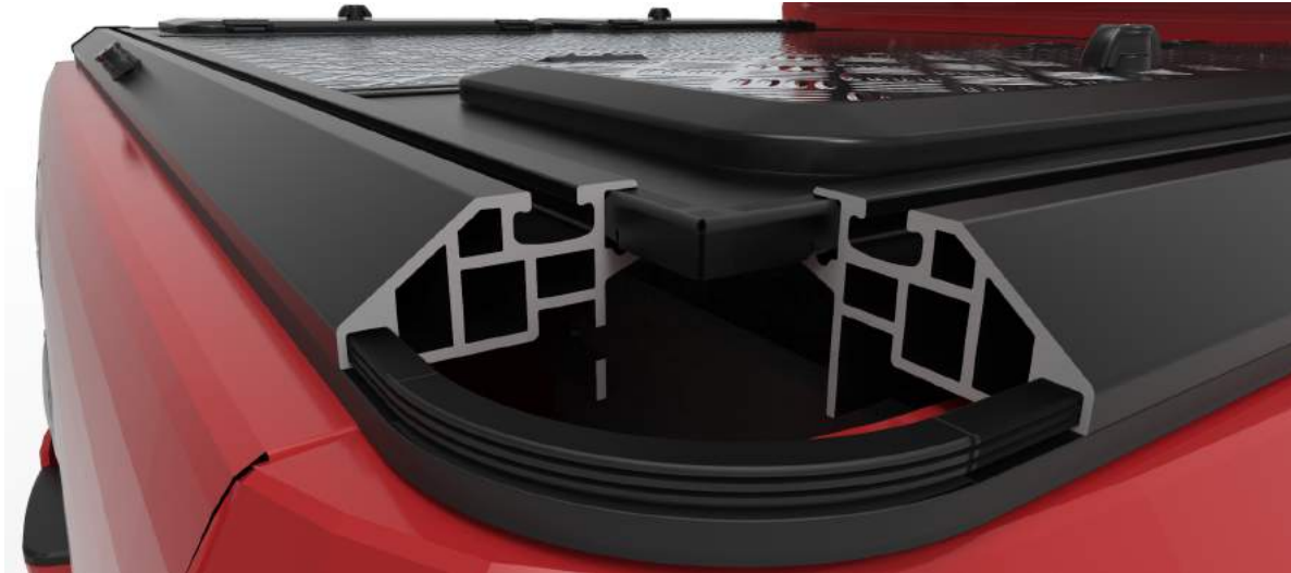
Figure 7.6: The U-shaped Side Sheet mounted to the Outer Profiles.
