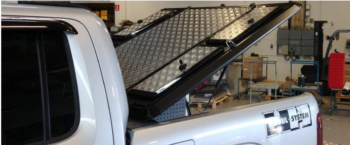
Figure 8.8: Modul-Cover in its opened position supported by gas springs.
