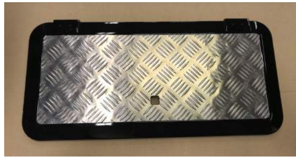
Figure 8.4: Top Plate glued to Upper Hatch Frame.
