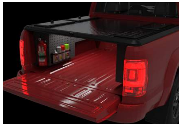
Figure 7.15: Illustration of integrated lighting installed.
