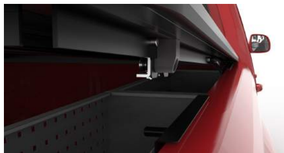
Figure 7.13: The locking system viewed from the outside of the pickup.
