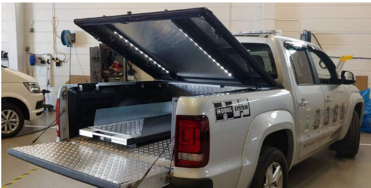
Figure 8.9: Integrated lighting in the prototype.
