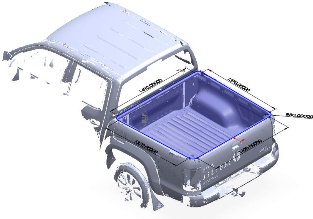
Figure 5.2: 3D-scan of a Volkswagen Amarok with measurements.
