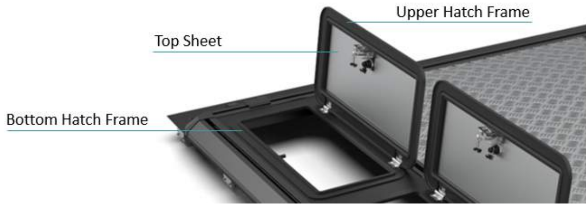
Figure 7.7: Illustration of one hatch with parts named.
