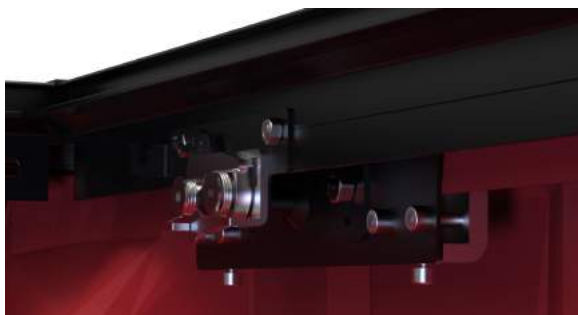
Figure 7.12: The locking system viewed from inside of the pickup bed.
